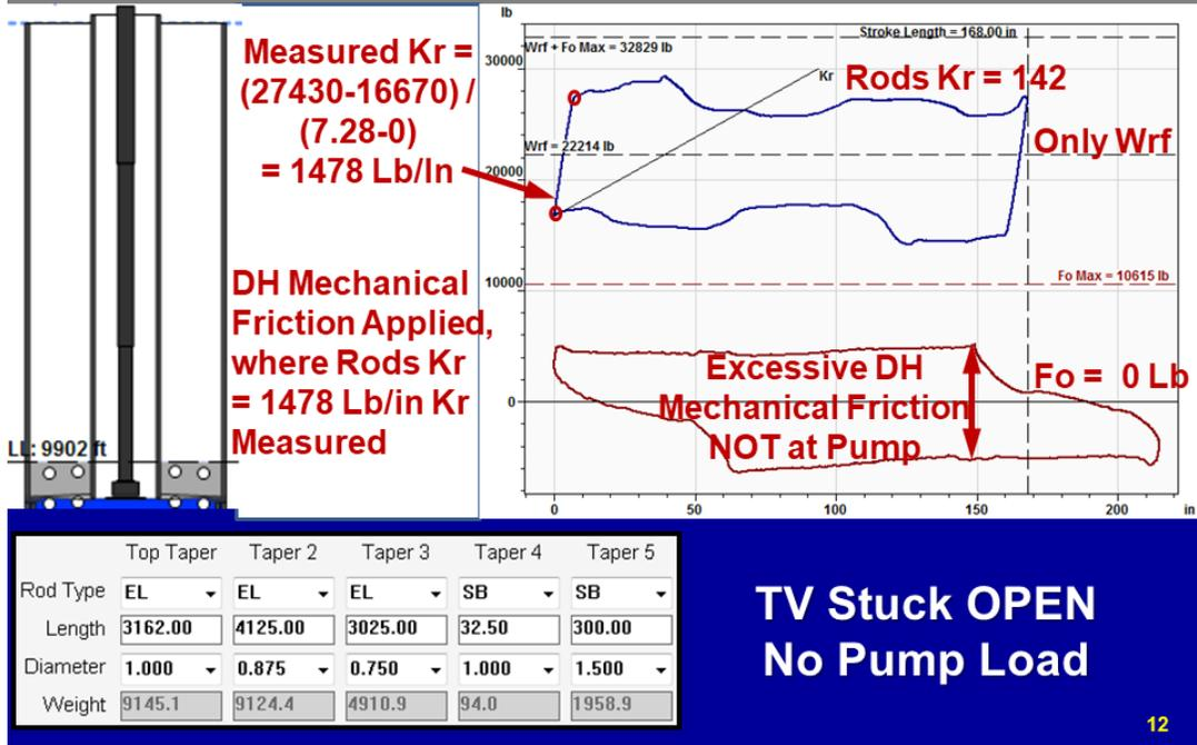
**Figure 6:** Plot of a dyno card on a running well exhibiting the transition from static to dynamic friction. The depth and relative magnitude of this friction can then be calculated from the rod properties. (Rowlan, Taylor, & Skinner, 2019)
