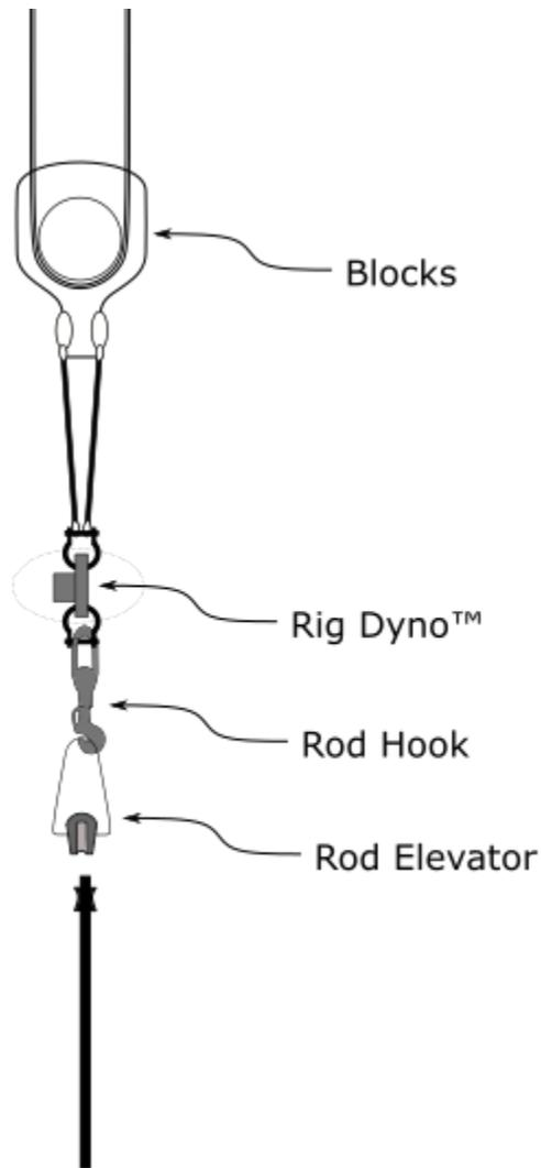
**Figure 4:** The general configuration of the sensing device on a typical workover rig when running rods. Ordinarily, the rod hook is shackled directly to the bails. The prototype device is inserted into this connection with a second shackle. Other load sensing devices, such as a directly instrumented rod hook or shackle, could simplify the installation.
