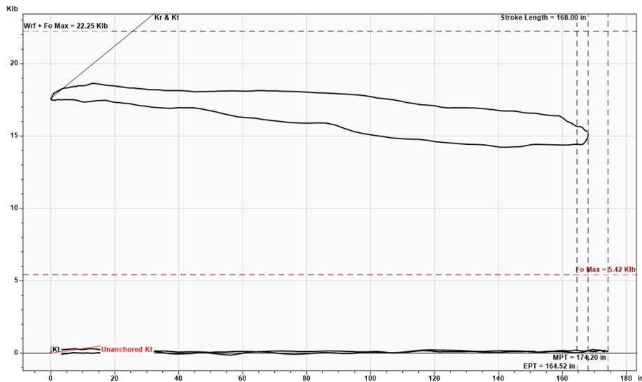
**Figure 3:** The pump dyno card of a deep rod part, in the absence of friction, would be a perfectly flat line with zero load. In practice and following the Gibbs Conjecture, the calculated load at the bottom of the rod-string is non-zero and indicates friction acting somewhere along the rod-string. Other factors such as incorrect damping or incorrect rod count can also impact that load. (Image source: Ecometer TAM example “RodPart\_NoPlunger”)
