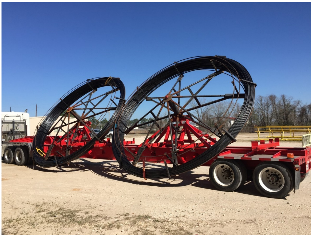
Figure 5: Double reel transport trailer rig for continuous rod installation – close up
