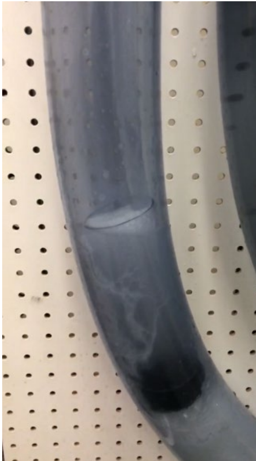
FIGURE 16 – SEPARATOR’S COLLECTOR FULL OF LIQUID UPON FLOW LOOP SHUT DOWN DEMONSTRATING ALMOST ALL GAS SEPARATION IS OCCURING ABOVE THE COLLECTOR IN THE “NO ANNULUS” SEPARATION REGION (DUE TO LIQUID FALLBACK AND NOT GAS BUBBLE RISE VELOCITY)
