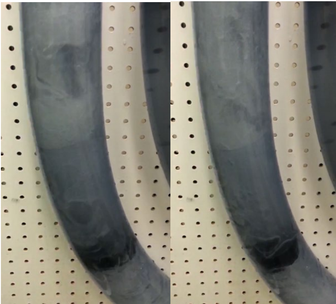
FIGURE 15 – FLOW LOOP TESTING SHOWING LIQUID FALLBACK COMENCING FROM IN SEPARATION REGION AND THEN DOWN INTO THE SEPARATOR'S UPWARD FACING COLLECTOR INTAKE
