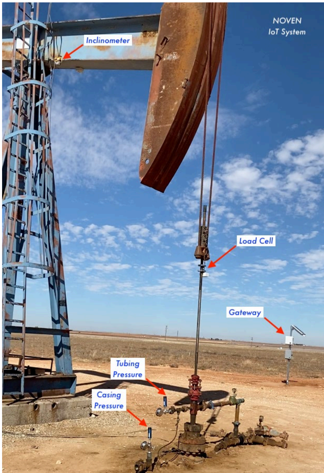
Figure 3 Typical IoT System Installation for SRP Wells
