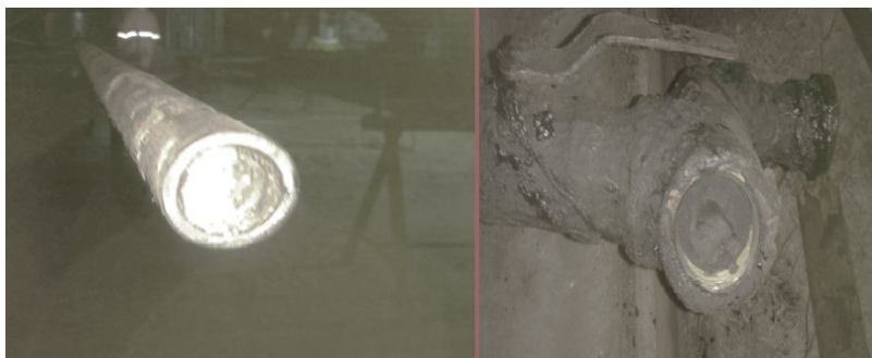
FIGURE 6: TYPICAL ISSUES WITH HEAVY PARAFFIN ON WELL PP
