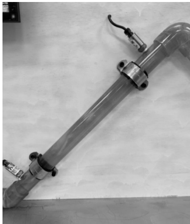
Figure 11: Plug Flow in 45° Inclined Section
