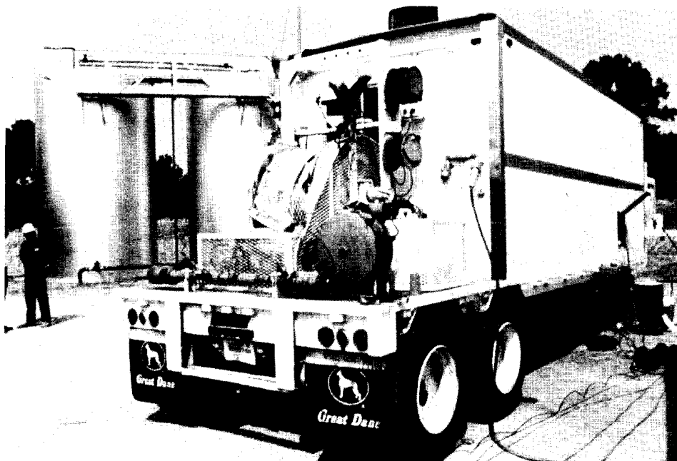
Rear view of DAT Trailer. Shown is wireline spool shieve and grease head.
