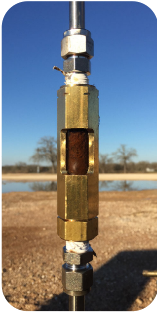
Figure 8 – Clear sight glass on slip-stream. These allow a pumper to visually see if the slip-stream is properly operating and approximate how much fluid is slipping back downhole.
