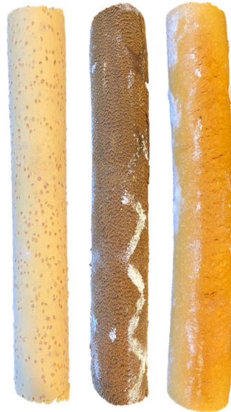
Figure 4 – Solid Time-Released Chemical Subs. The solid chemical sticks are inserted into chemical subs on bottom of the tubing string and they time-release into the produced fluids. Diagram images from Odessa Separators and images of solid chem sticks from Freedom Technologies (which are two providers of this technology). Chem sticks (from left to right): scale inhibitor, corrosion inhibitor, and paraffin inhibitor.
