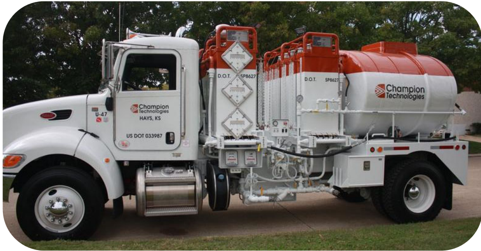
Figure 1 – Truck Treater (for batch chemical treatment). Truck carries tanks of various chemicals (in the front compartments) and a water tank on back that is loaded with produced water to flush the chemicals downhole.
