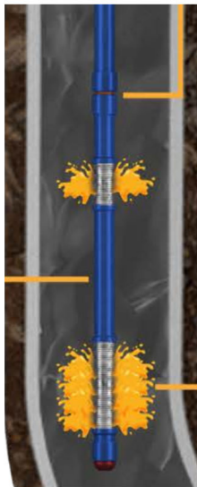
Figure 4 – Solid Time-Released Chemical Subs. The solid chemical sticks are inserted into chemical subs on bottom of the tubing string and they time-release into the produced fluids. Diagram images from Odessa Separators and images of solid chem sticks from Freedom Technologies (which are two providers of this technology). Chem sticks (from left to right): scale inhibitor, corrosion inhibitor, and paraffin inhibitor.
