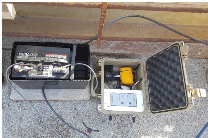
Figure 3 – RAM connected to external battery and Nitrogen supply for long term operation.
