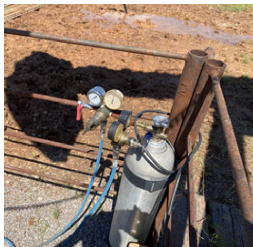
Figure 3 – RAM connected to external battery and Nitrogen supply for long term operation.
