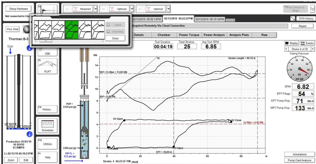
Figure 8 – Remotely acquired Dynamometer Record via Cloud Connection
