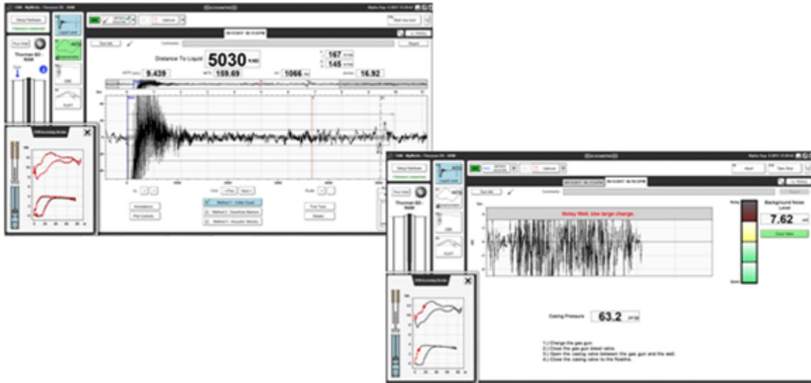
Figure 9 – Simultaneous fluid level and dynamometer remote acquisition
