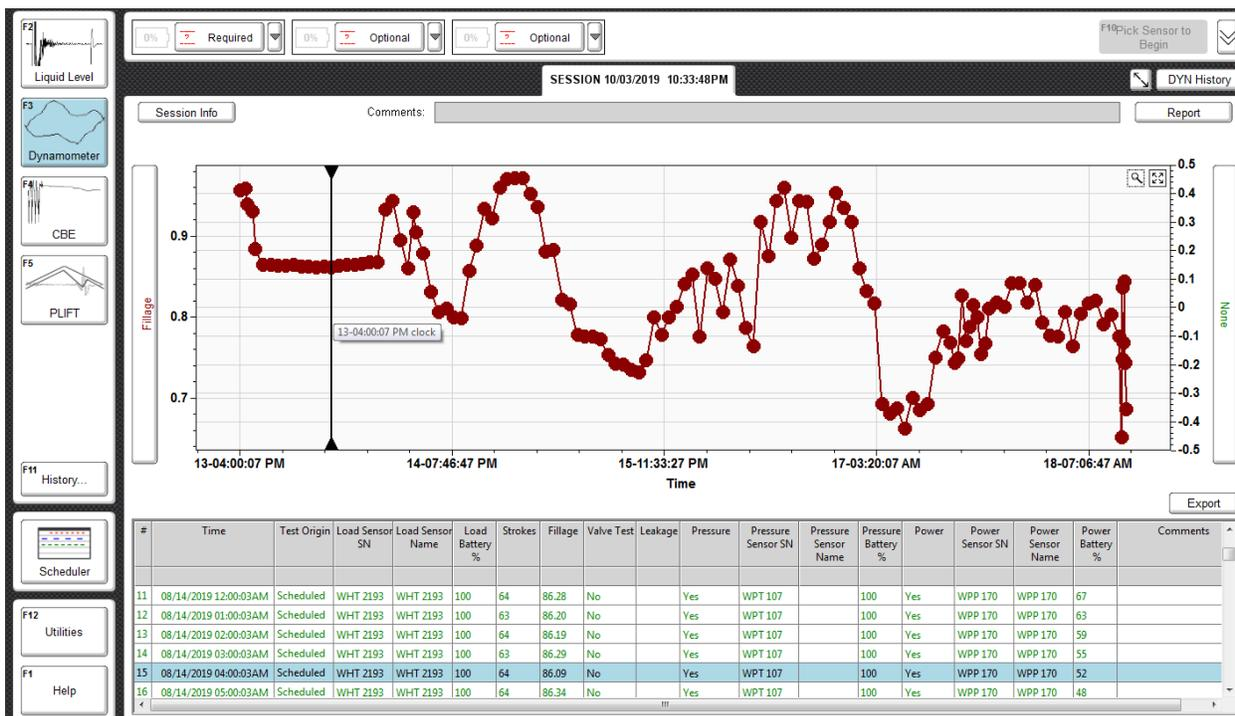
Figure 16 – Dynamometer Scheduled Acquisition during 5 Days showing Hourly Variable Pump Fillage
