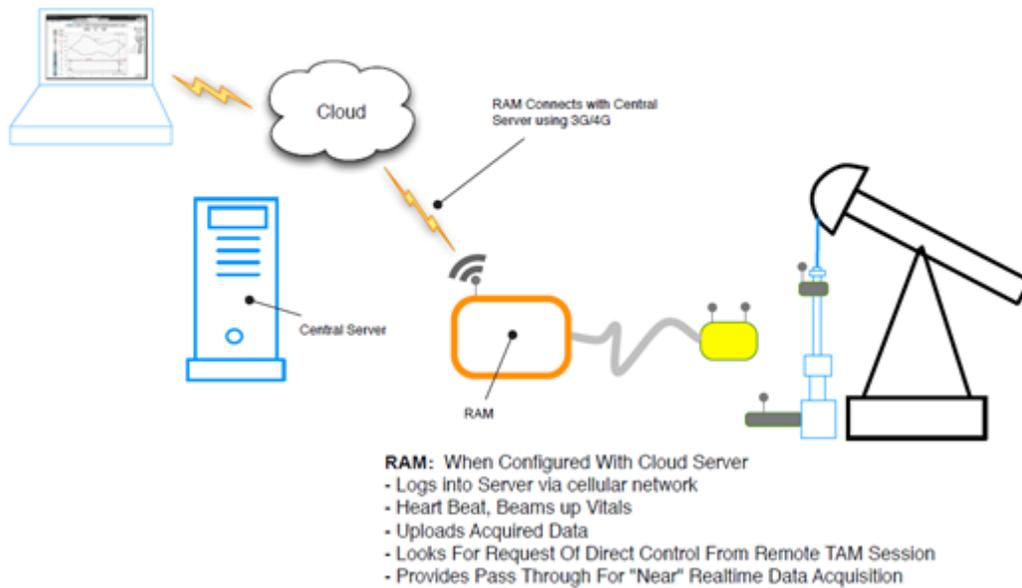
Figure 5 – Cloud Based Operation
