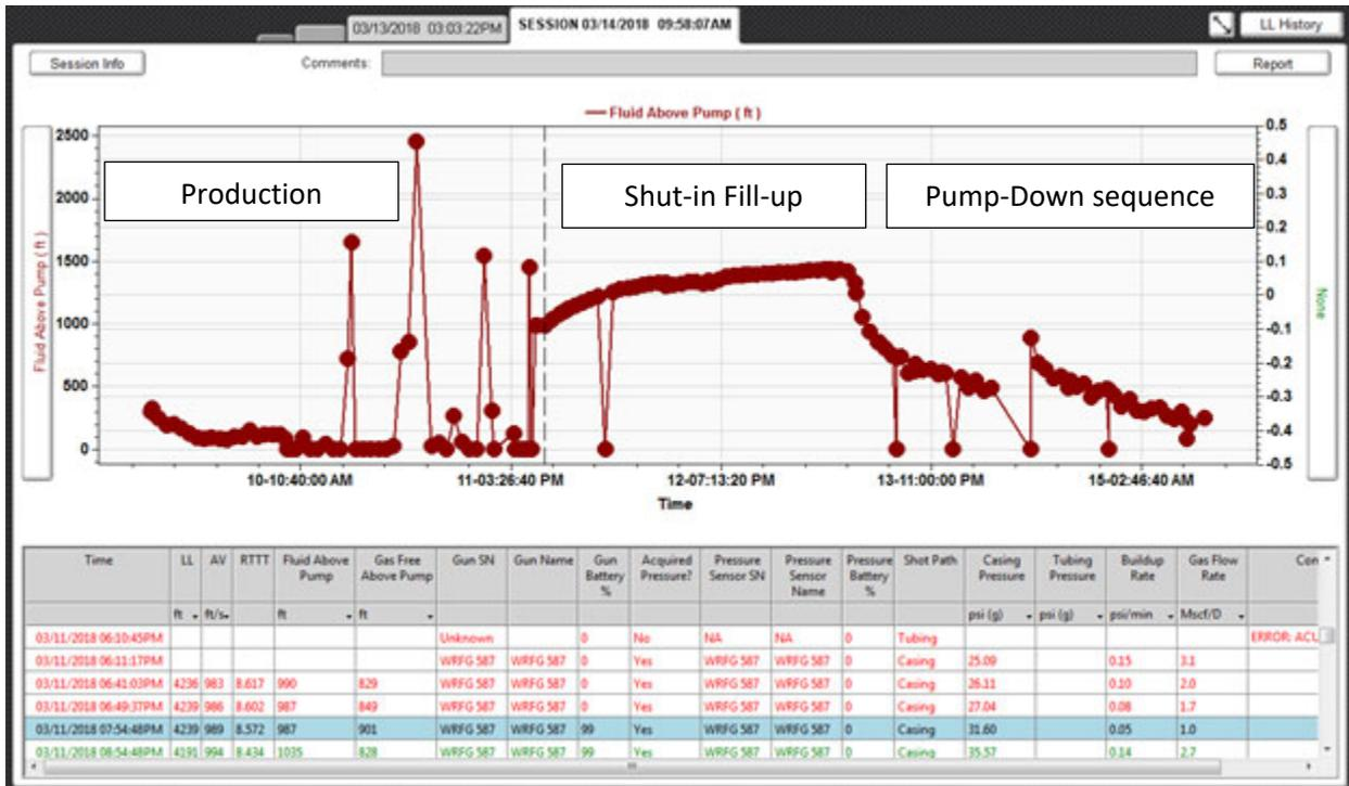
Figure 17 – Fluid Above Pump vs. Time Acquired automatically with RAM Schedule
