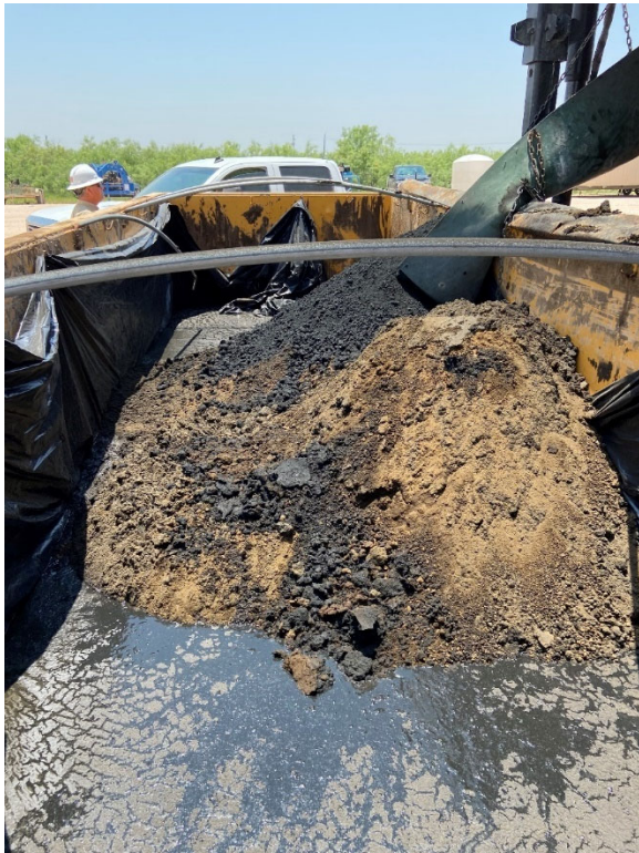
Figure 7: Downhole material cleaned out of the lateral
