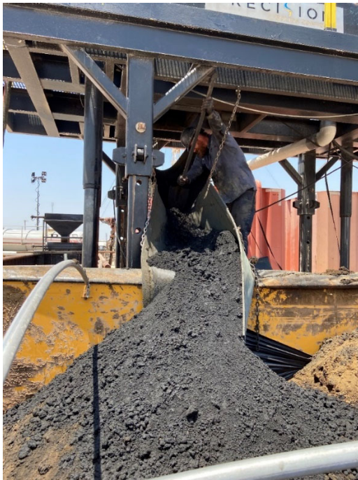
Figure 8: Downhole material cleaned out of the lateral
