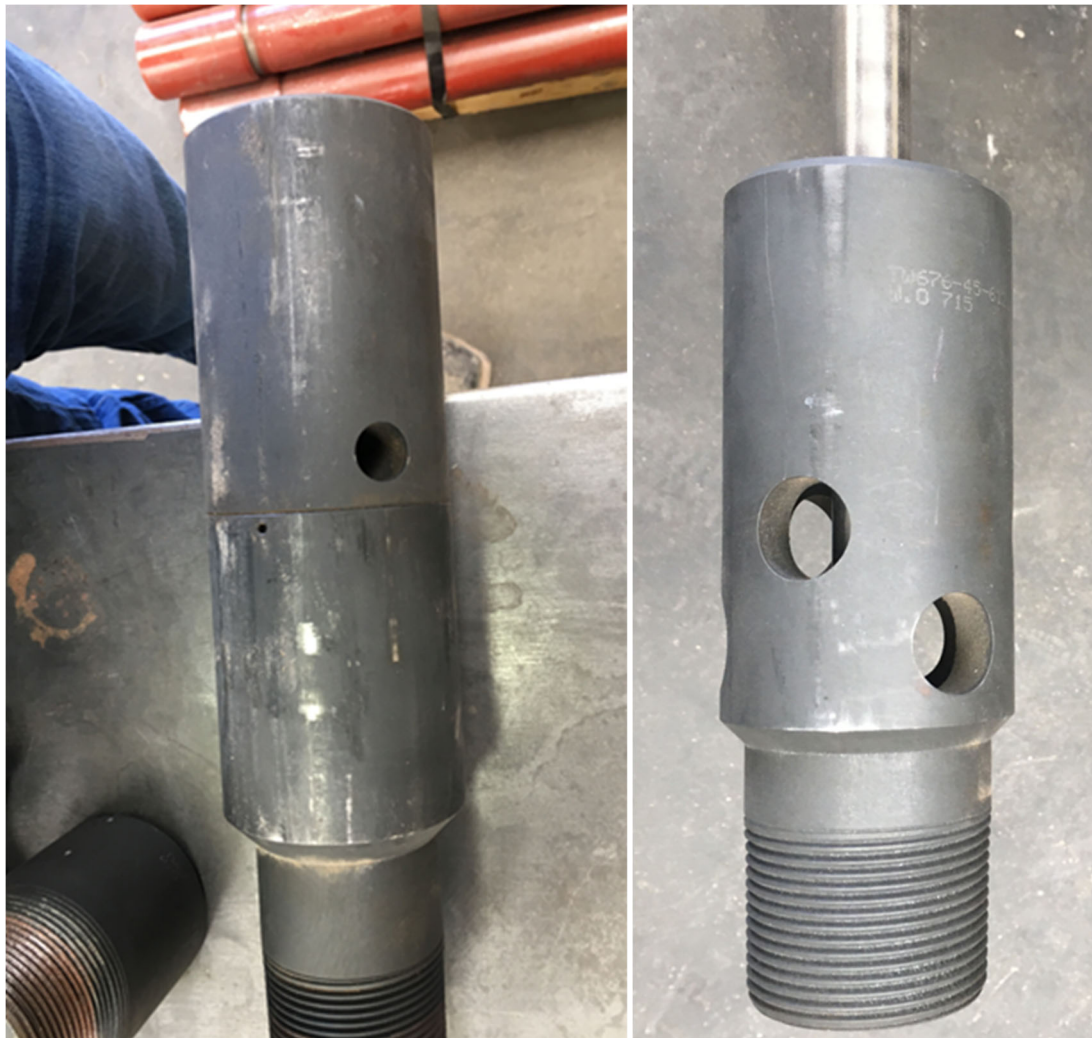
Figure 5: Sample subs used in pilot downhole equipment design
