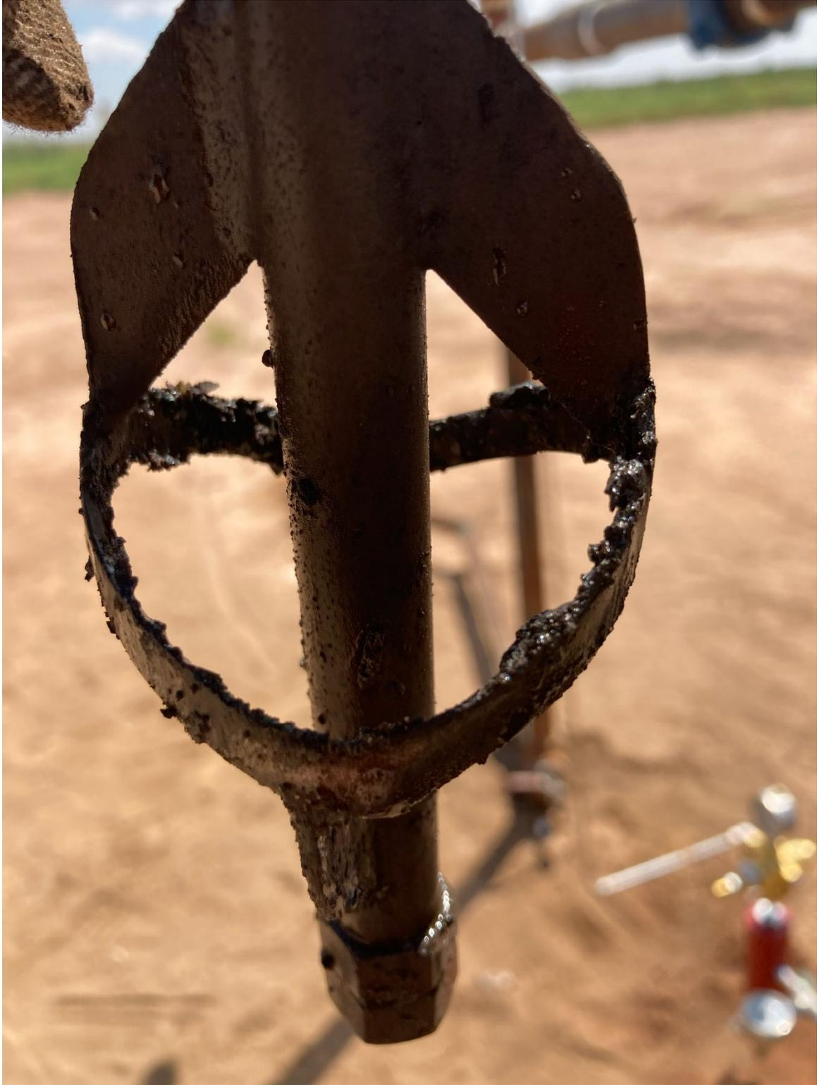
Figure 1: Knife before tripping in the hole through slickline.
