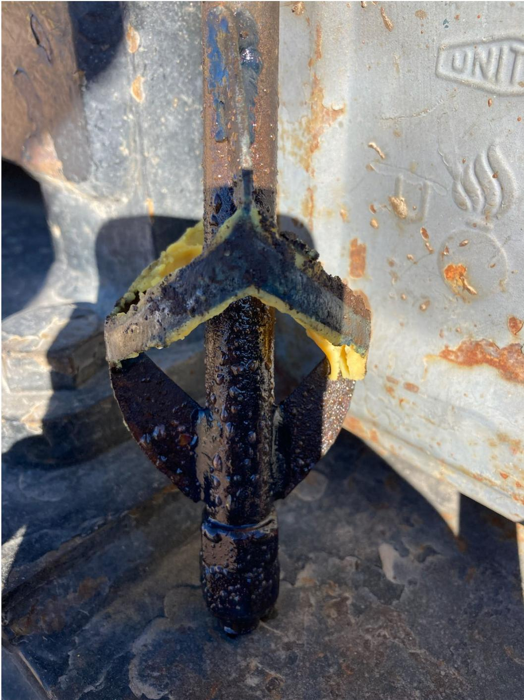
Figure 2: Knife showing small paraffin traces after tripping in to the hole through slickline.
