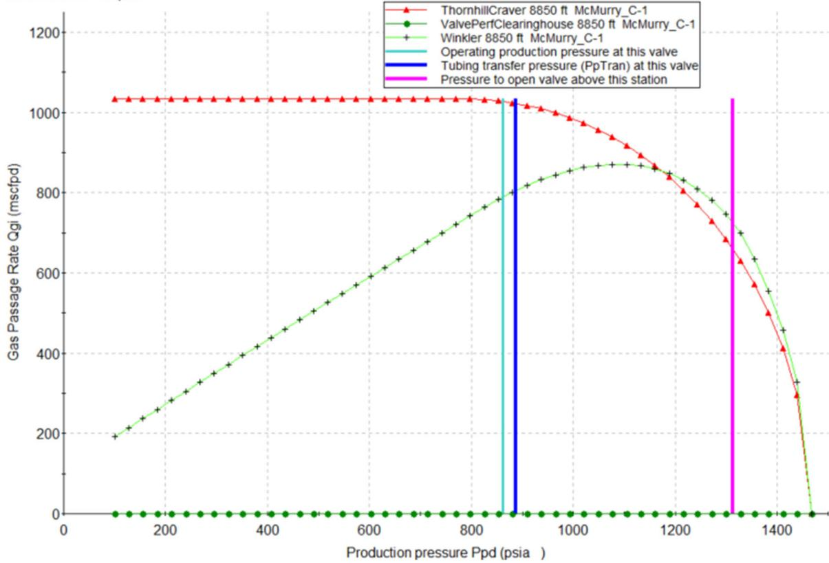
Figure 6: Valve performance relationship of the unloading valve.
