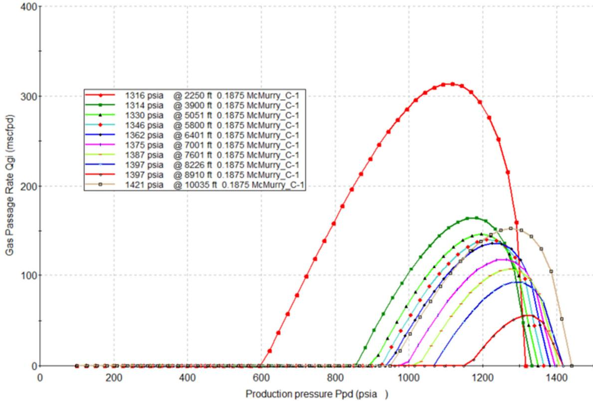
Figure 7: Spread of gas injection rate through all the 16 ports gas lift valve in this casestudy.
