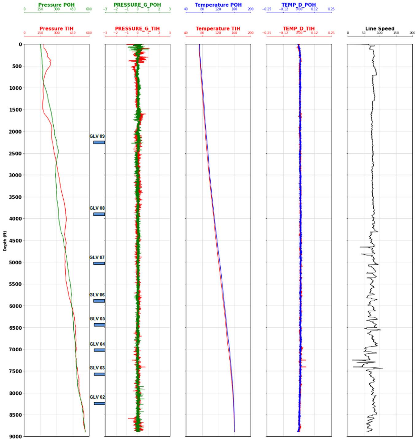
Figure 4: Continuous Pressure-Temperature Survey of the flowing well.
