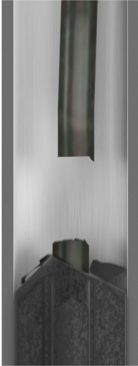
Figure 3. Rod Part at Rod Guide.
