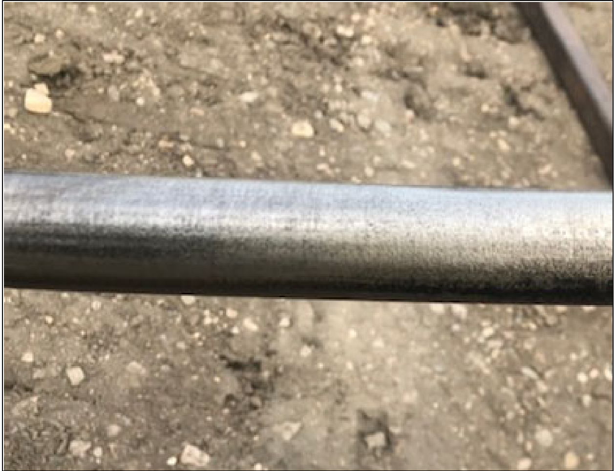
Figure 12 - Uncoated section exhibited wear near coated section (22 weeks)
