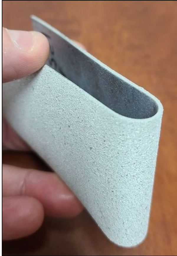
Figure 8 – Coated test panel bend testing
