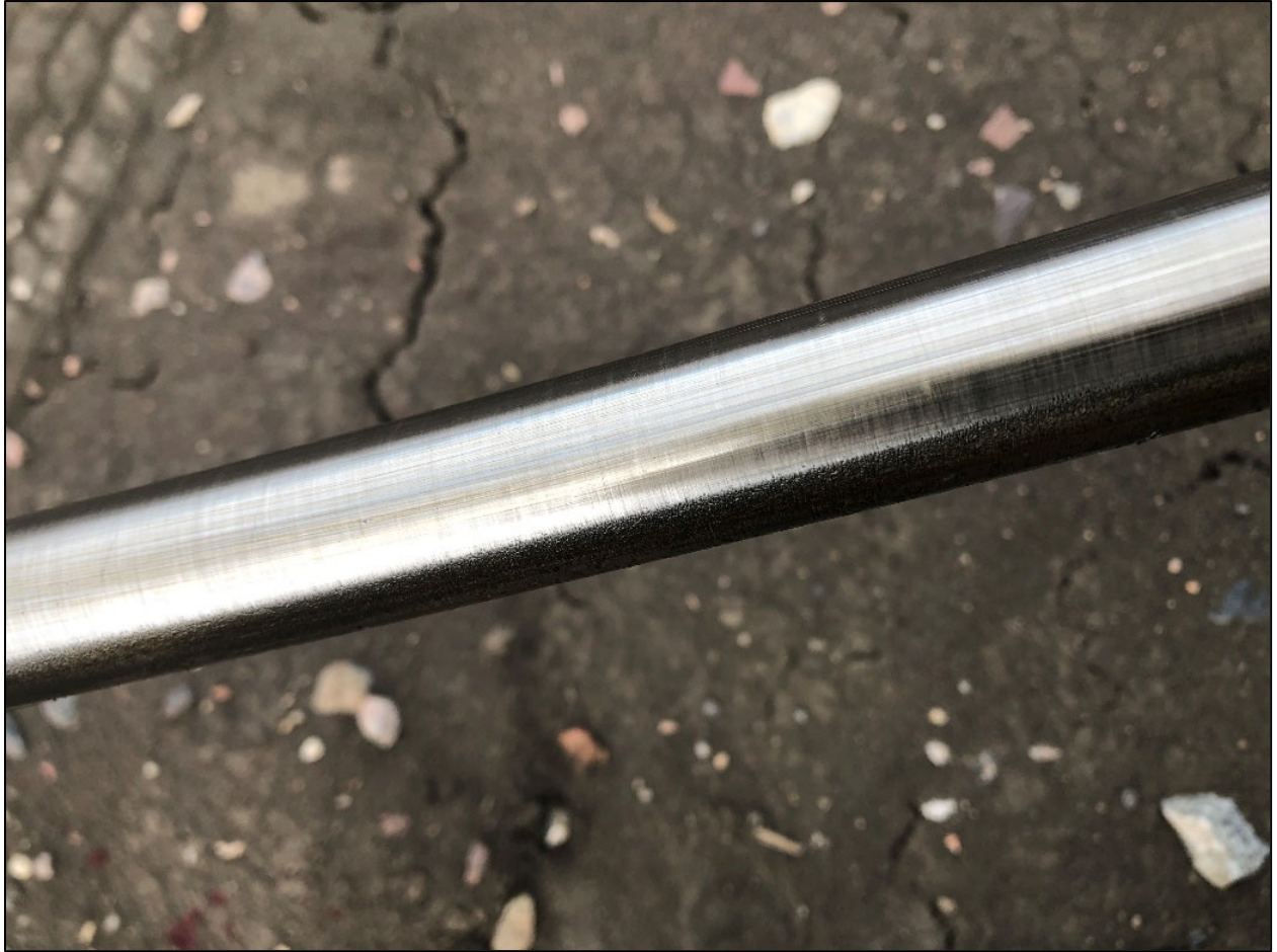
Figure 13 - Coated section exhibited light wear (22 weeks)
