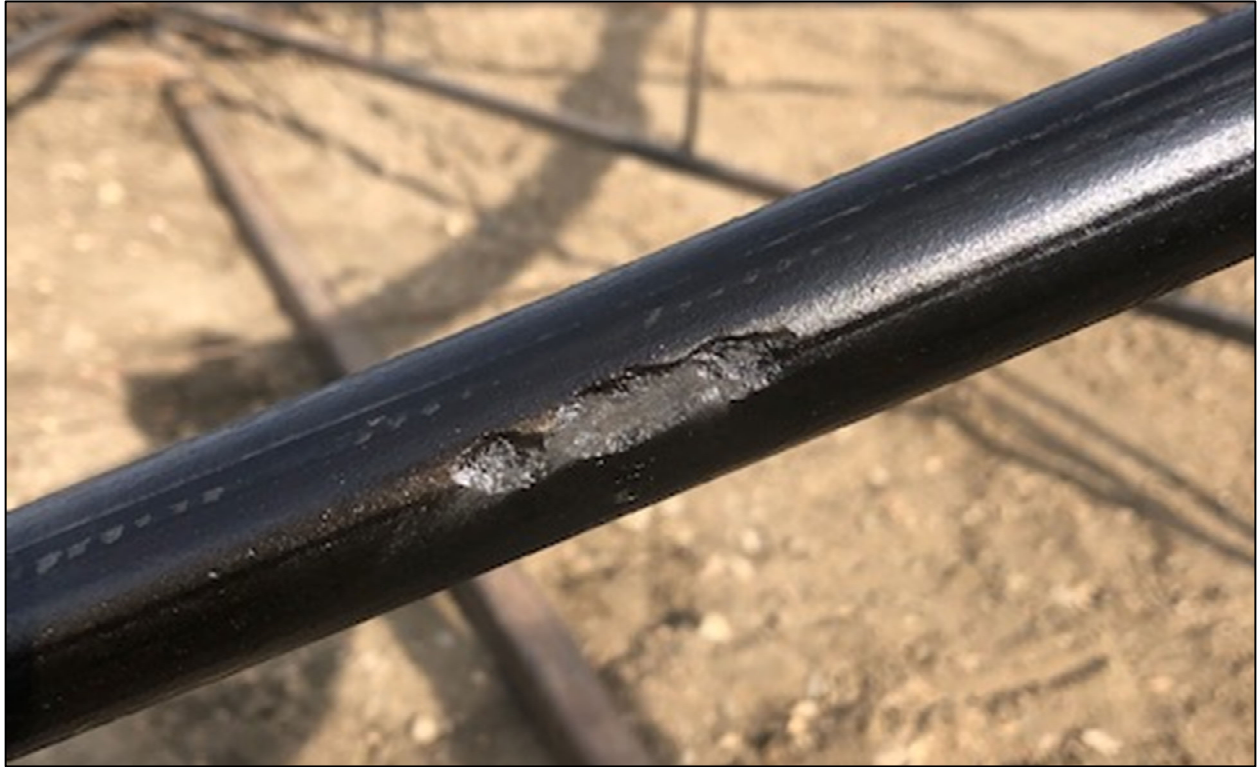
Figure 11 - Uncoated rod exhibiting corrosion damage at 22 weeks
