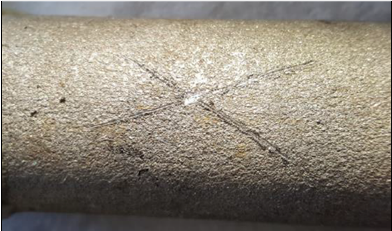
Figure 6 – X-cut evaluation of coating corrosion test
