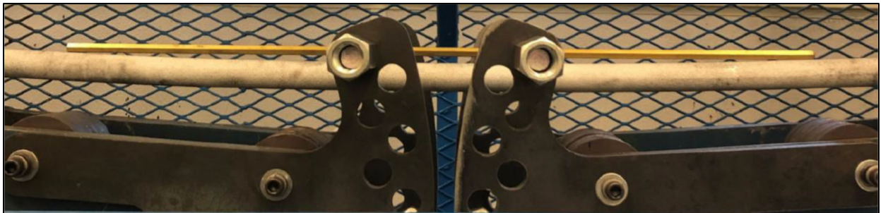
Figure 9 – Coated rod rotating bend testing (brass rod used to demonstrate rod curvature)
