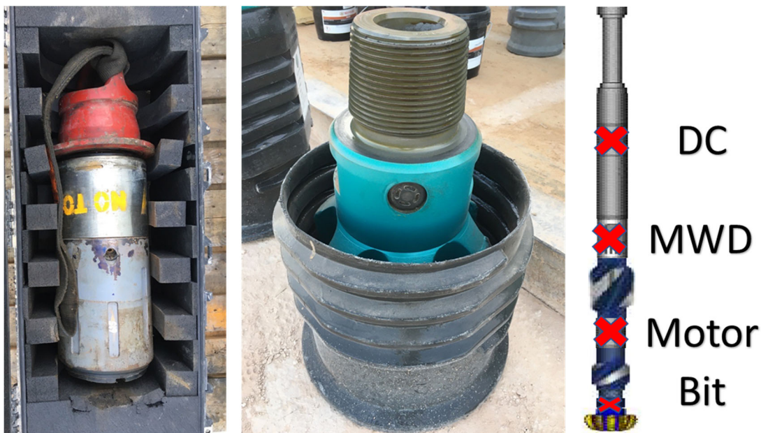
Figure 20 - The project BHA recorded 100 Hz data with sensors installed at bit and subs above the mud motor and in the drill collars.
