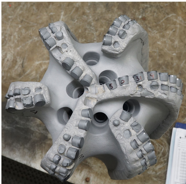
Figure 31 – 2 nd trial well bit dull. Severe shoulder wear flats, delamination, and trim cutter damage. Tungsten carbide DOCC engaged at 0.35 in/rev and worn down.
