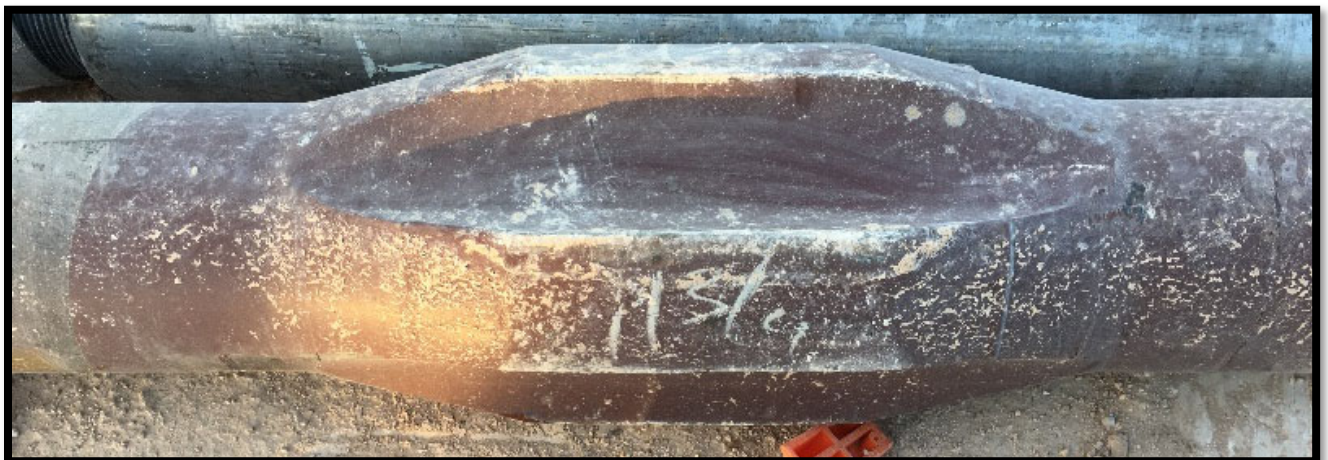
Figure 27 – 11 3/4" Straight integral blade stabilizer used on all wells except for the trial well 3. No observable damage, the IBS also measured gauge post-drill.
