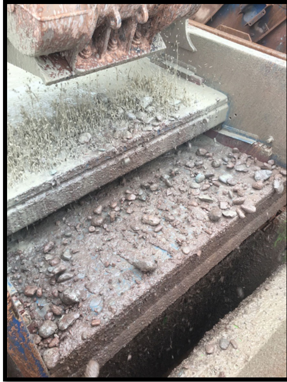
Figure 12 – A bit did not cut the rocks on the shaker screen. Fine wetted rock powder is expected from the drilling process. The large rocks are cavings. Angular or rounded edges would confirm the borehole instability severity. Mud weight should be raised immediately.
