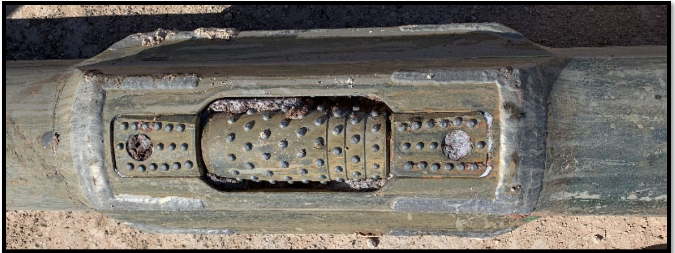
Figure 26 – Trial well 3 roller reamer post-drill. Sealed bearing retention system worked effectively. Note the wear on the carbide buttons but no unusual tool integrity damage.
