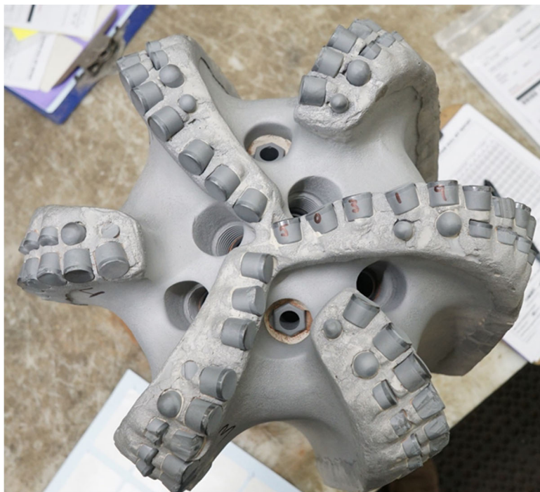
Figure 30 – 1 st trial well bit dull. Severe shoulder wear flats, delamination, and trim cutter damage. Original default DOCC set a 0.70 in/rev did not engage.
