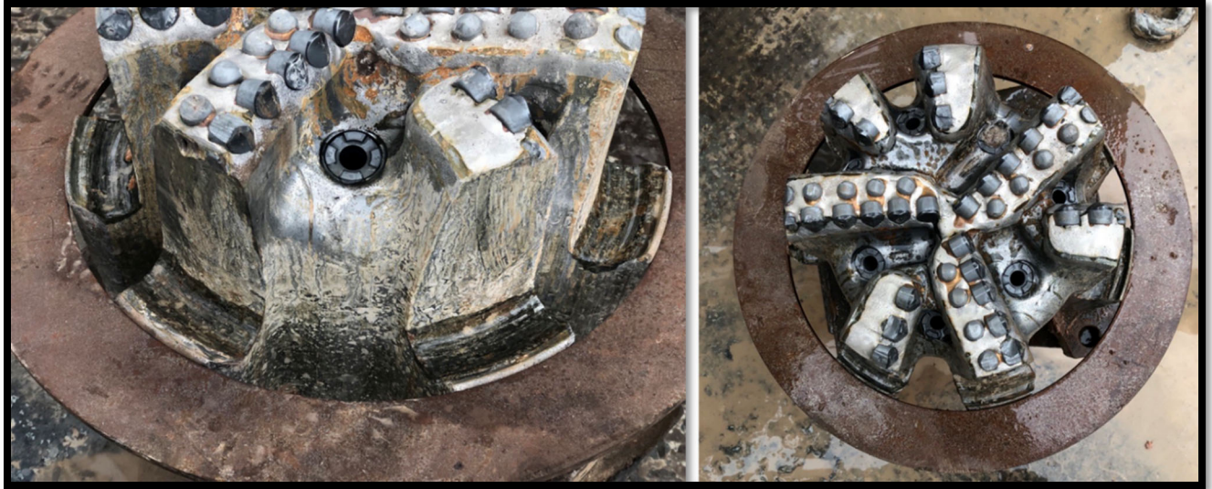
Figure 10 – The bit in Figure 9 experienced a shoulder ring out from severe stick slip. The lack of cone cutter damage indicates full stick slip was not the leading cause of damage.
