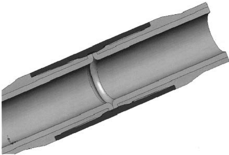
Figure 1 - Premium Connection with Thermoplastic Liner
