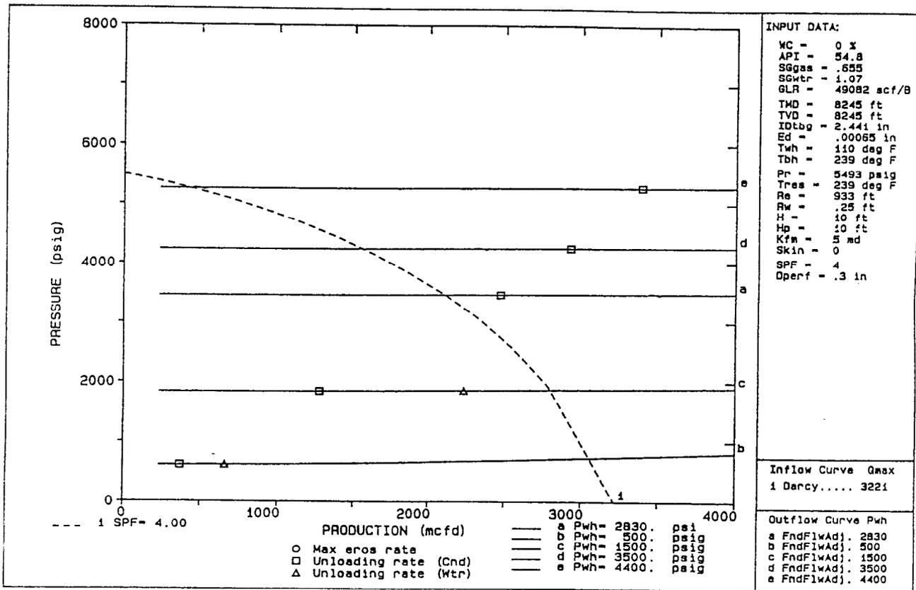
Figure 2 - Lobo gas well-systems analysis plot
