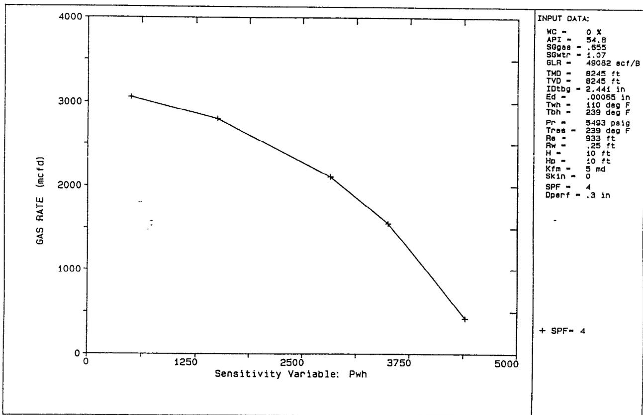
Figure 3 - Lobo gas well-outflow sensitivity (gas rate vs. wellhead pressure)
