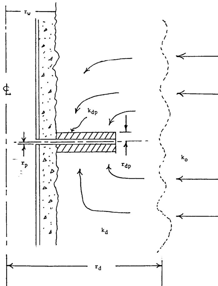
Figure 1 - Flow into a perforation
