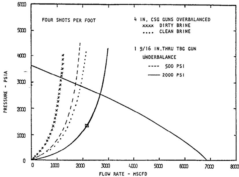
Figure 5 - Completion pressure drops for through-tubing and casing guns
