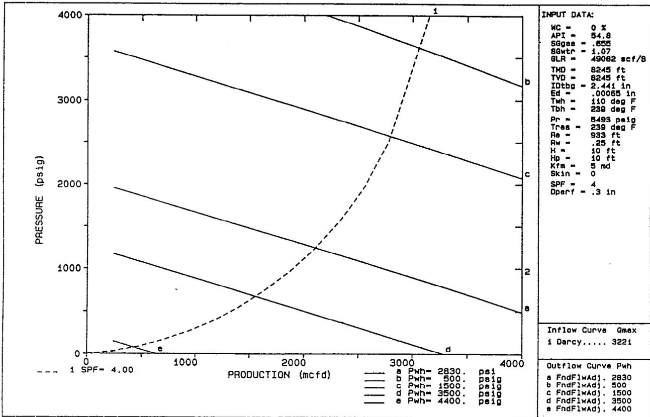
Figure 4 - Lobo gas well-differential curve (completion pressure drop)
