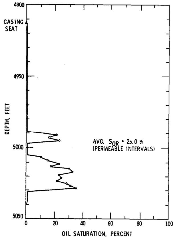
OIL SATURATIONS COMPUTED FROM THERMAL NEUTRON DECAY TIME LOGS RUN AFTER CORING, AFTER INJECTING SALT WATER, AND AFTER INJECTING ALCOHOL FOLLOWED BY SALT WATER, SAN ANDRES FIELD A, TEXAS
