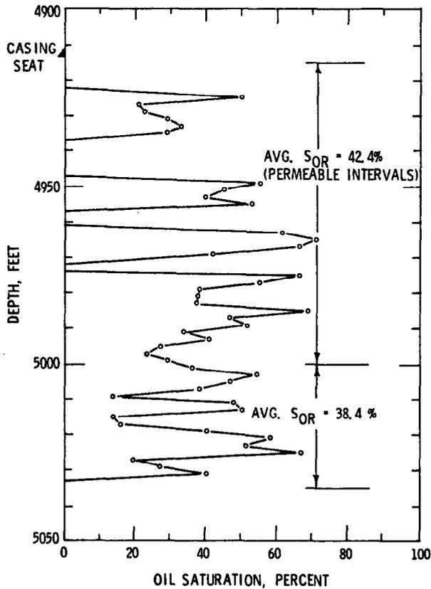
OIL SATURATIONS COMPUTED FROM THERMAL NEUTRON DECAY TIME LOGS RUN AFTER CORING AND SALT WATER INJECTION. SAN ANDRES FIELD A, TEXAS
