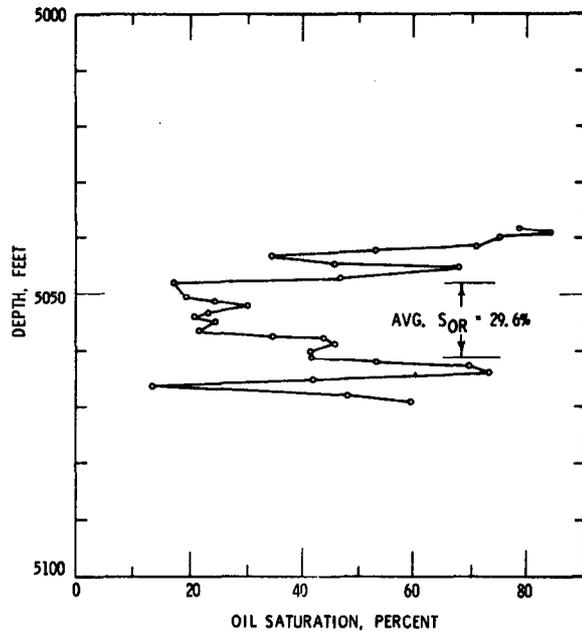
OIL SATURATIONS COMPUTED FROM THERMAL NEUTRON DECAY TIME LOGS RUN AFTER INJECTING SALT WATER AND FRESH WATER, MUDDY SAND, COLORADO
