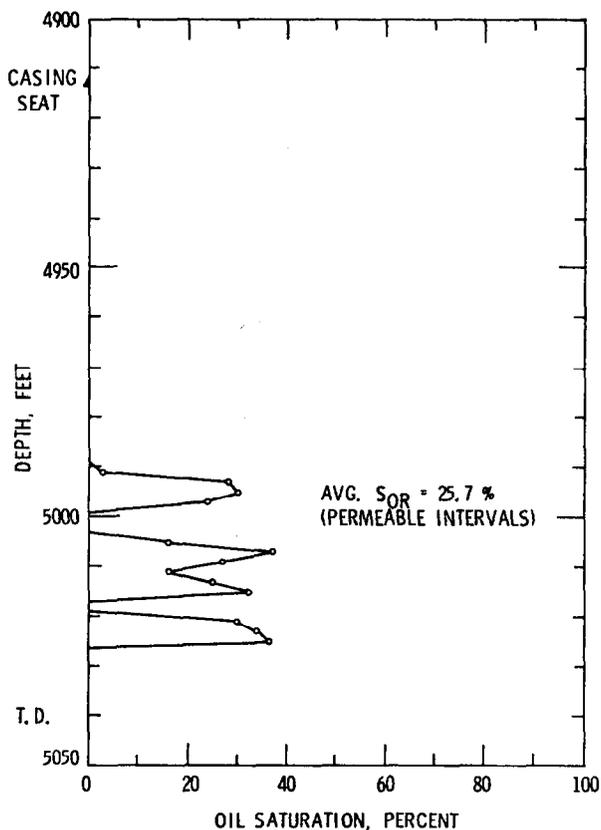
OIL SATURATIONS COMPUTED FROM INDUCTION LOG-INJECT-INDUCTION LOG PROCEDURE, SAN ANDRES FIELD A, TEXAS
