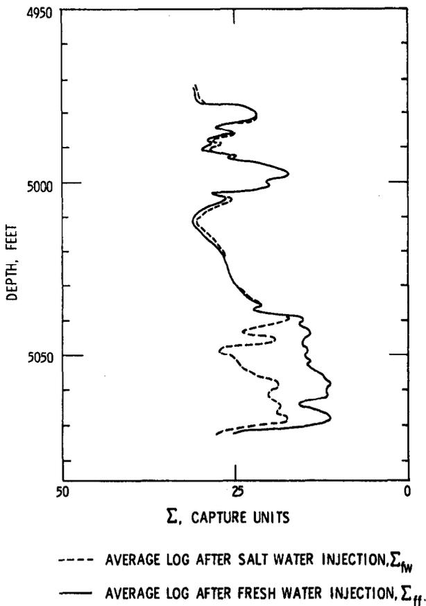
AVERAGE THERMAL NEUTRON DECAY TIME LOGS, MUDDY SAND, COLORADO
