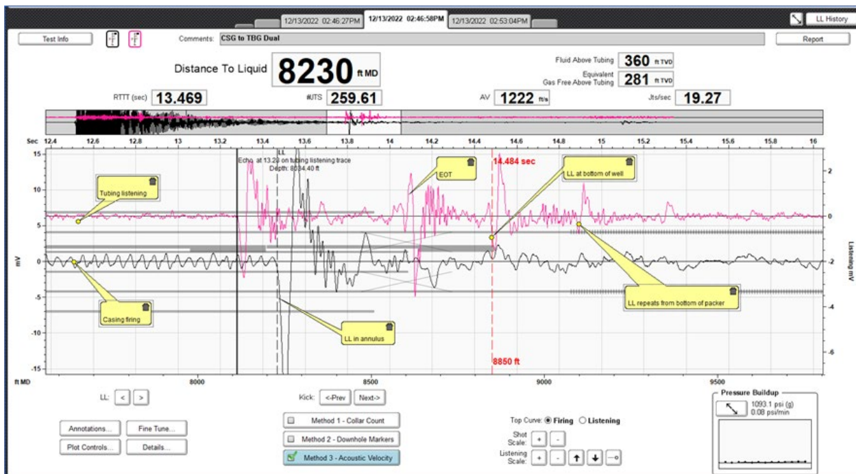
Figure 10 – Dual shot Casing Firing and Tubing Listening. Communication point at 8034 feet.
