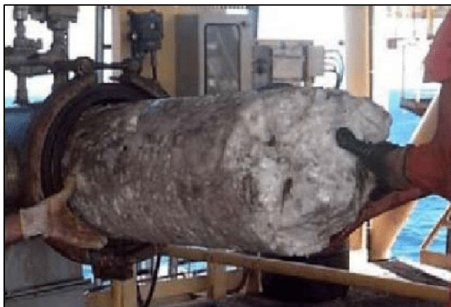
Figure 1 – Hydrate blockage in a pipe
