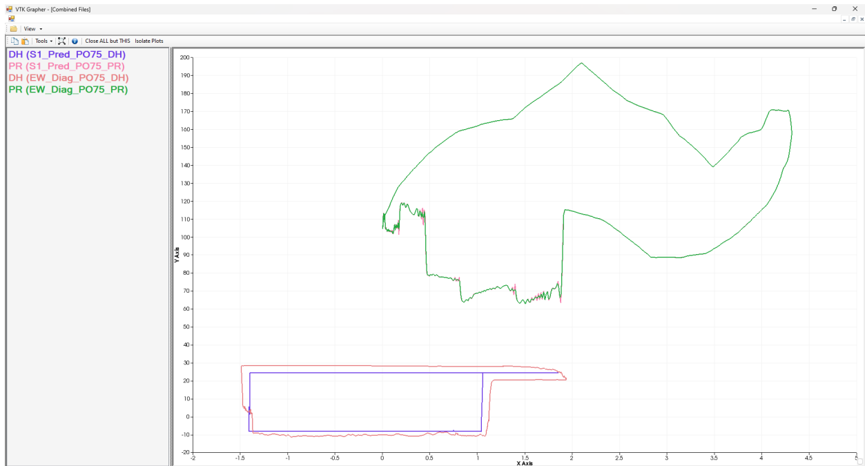
Figure 15 - If the EW trajectory is used in the diagnostic model, we get significant error in the estimation of the DH card.
