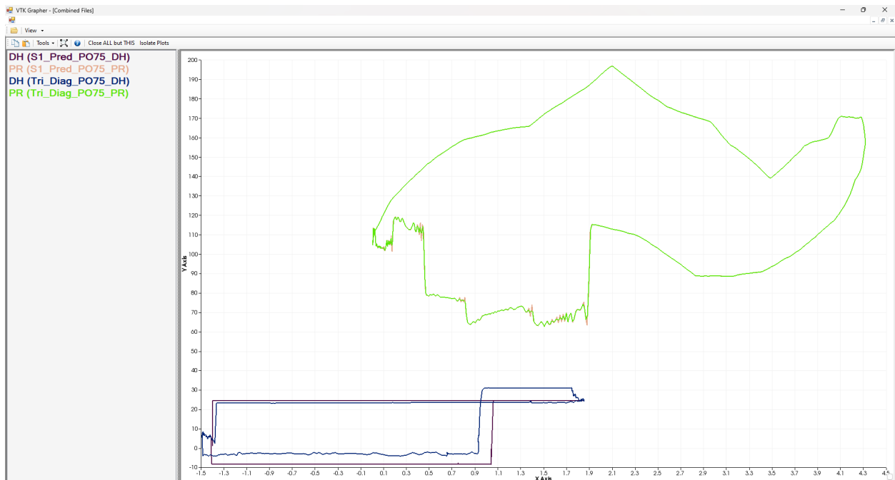
Figure 16 - Similarly, if the pseudo 3D “triangulated” trajectory is used in the diagnostic model, the estimation of the DH card is significantly off.
