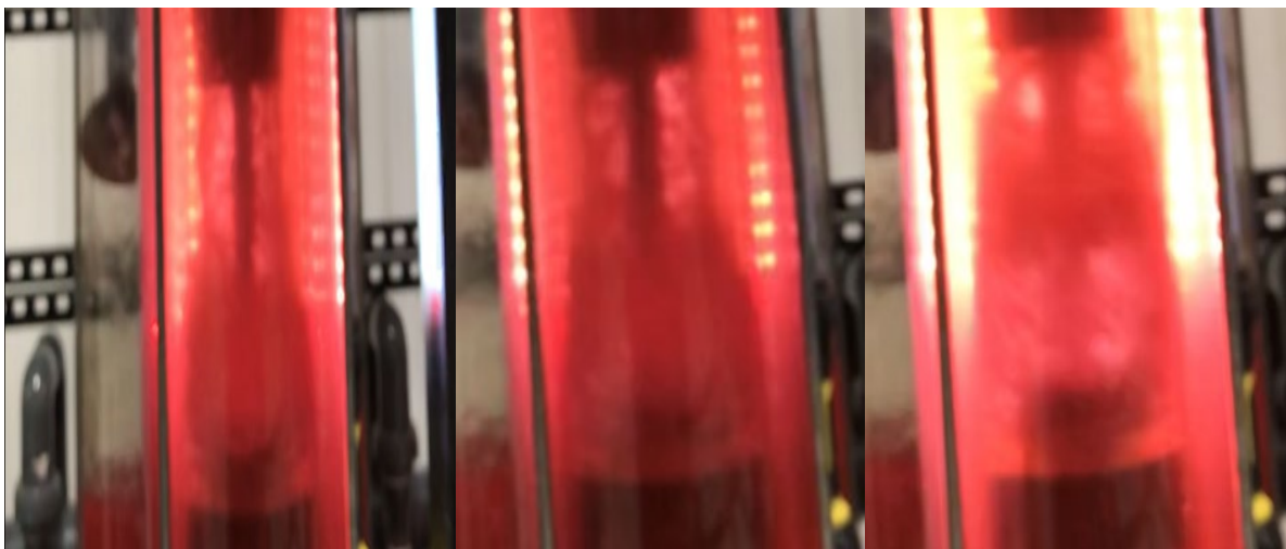
Figure 2 – Mixing and separating regions inside the vortex gas separator
