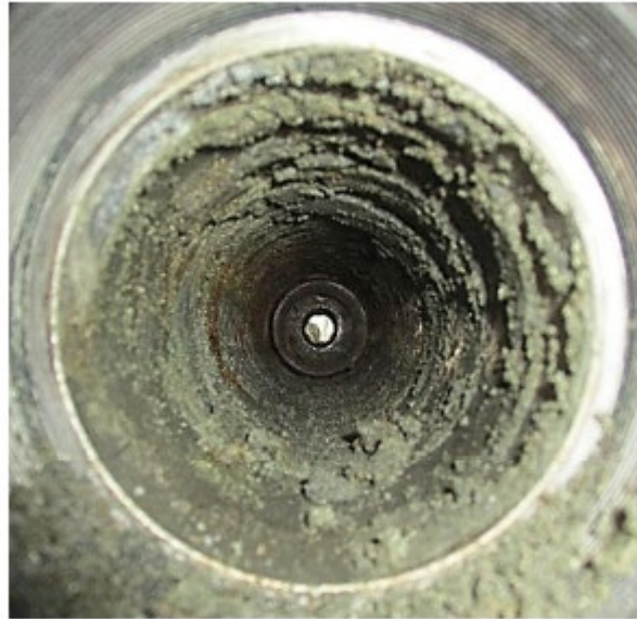
Figure 11- Pump plugged with solids
