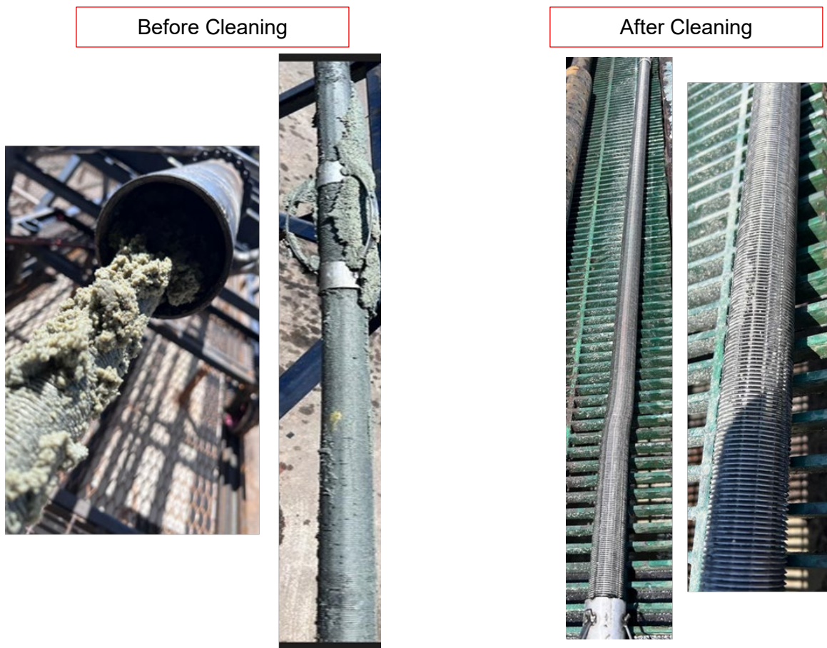
Figure 6 Inner string before and after cleaning process
