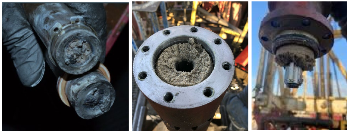
Figure 1 Problems caused by sand on ESPs
