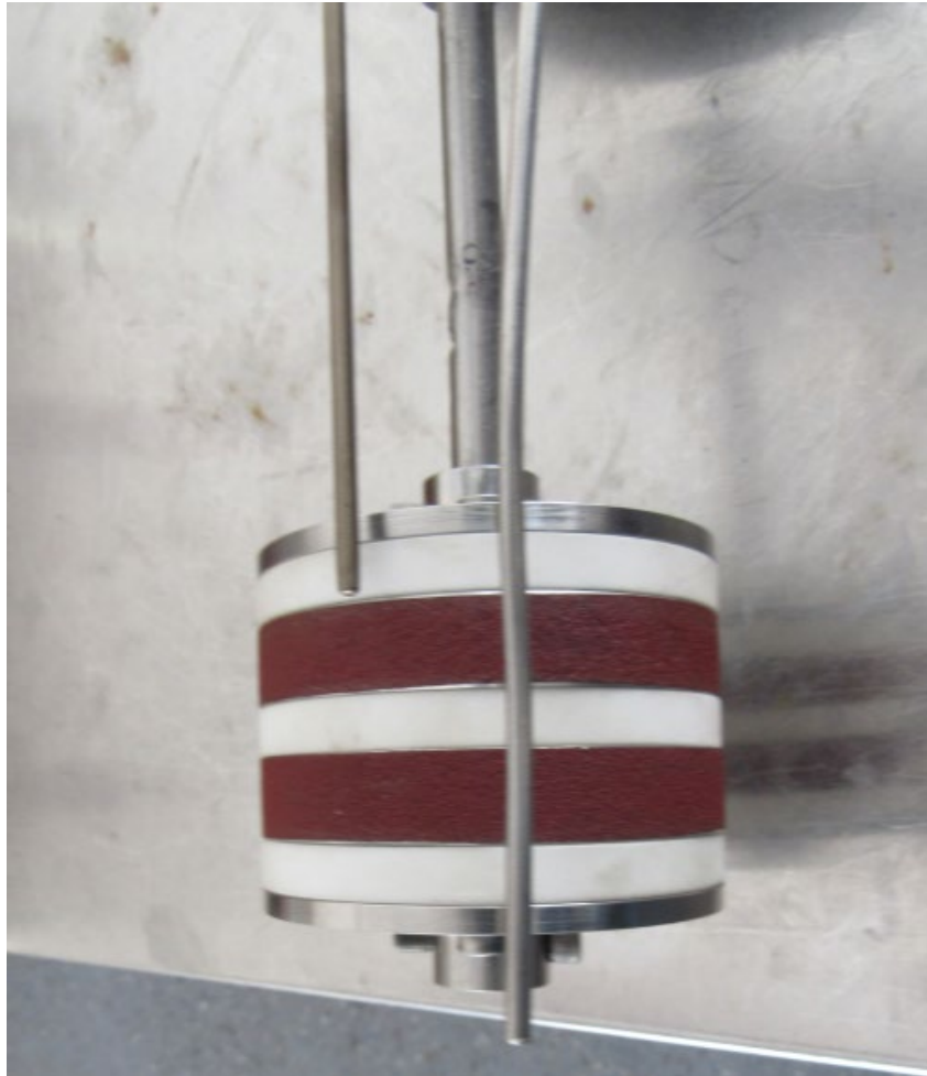
Figure 6 – Autoclave testing of a spray metal coating applied to 2 7/8" L80 tubing.
