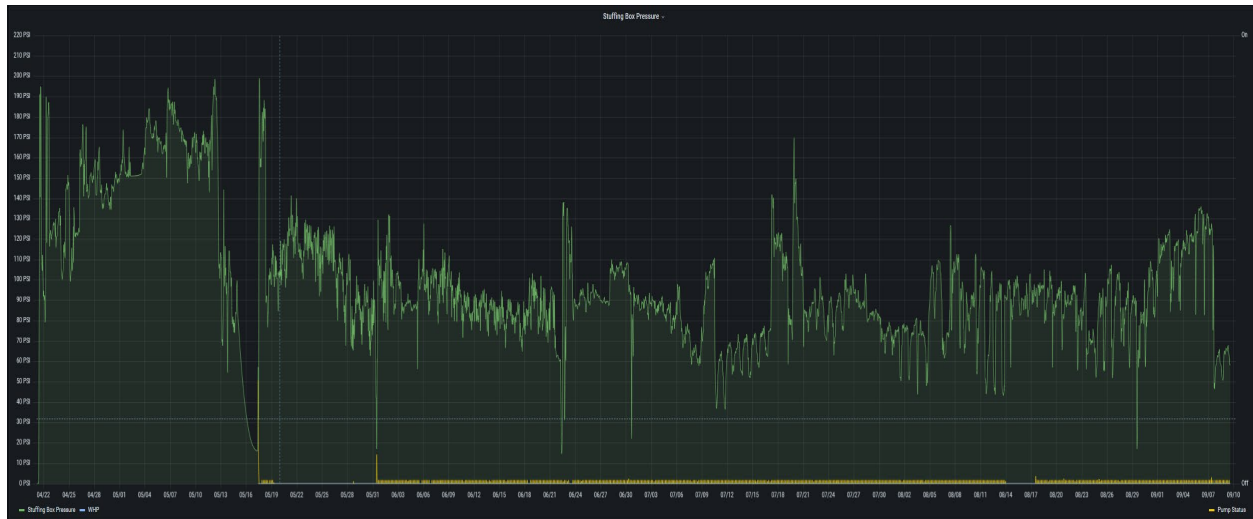
Figure 5 Internal stuffing box pressure for test period.
