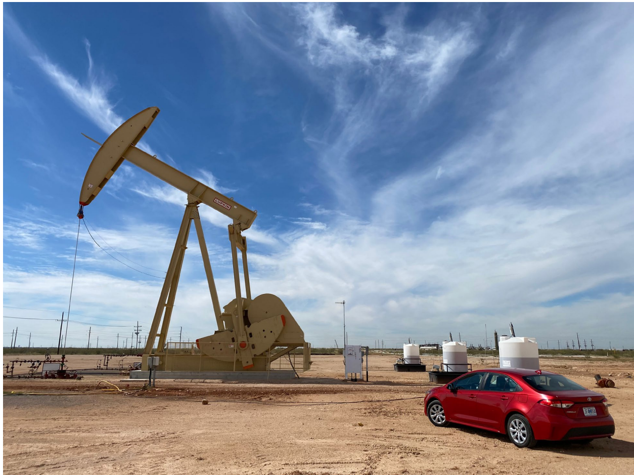
Figure 9—2560–500–320 conventional pumping unit next to a very small rental car.
