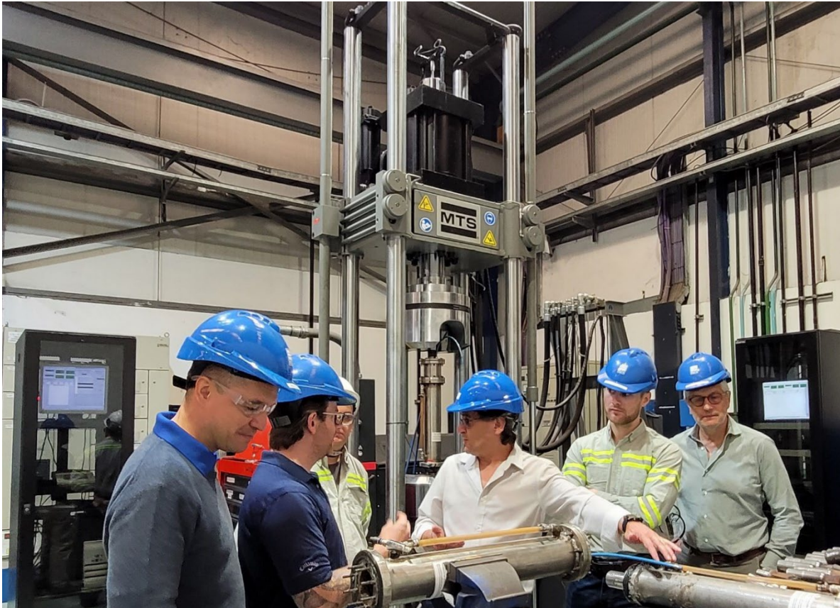
Figure 14 Corrosion fatigue testing machine and test chambers
