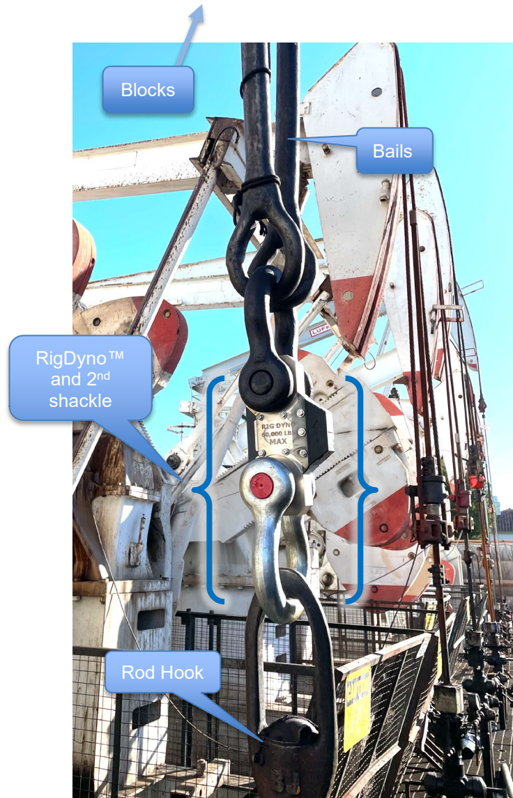
Figure 1: The RigDyno™ is placed in-line with the rod hook. A second shackle is required to complete the connection. Once installed, the load-cell observes all load placed below, on the rod hook. The sensor also determines position of the rod hook throughout the stroke. Because the load and position are gathered at the same physical location and time, they are directly suitable for use as inputs to an unaltered wave equation.
