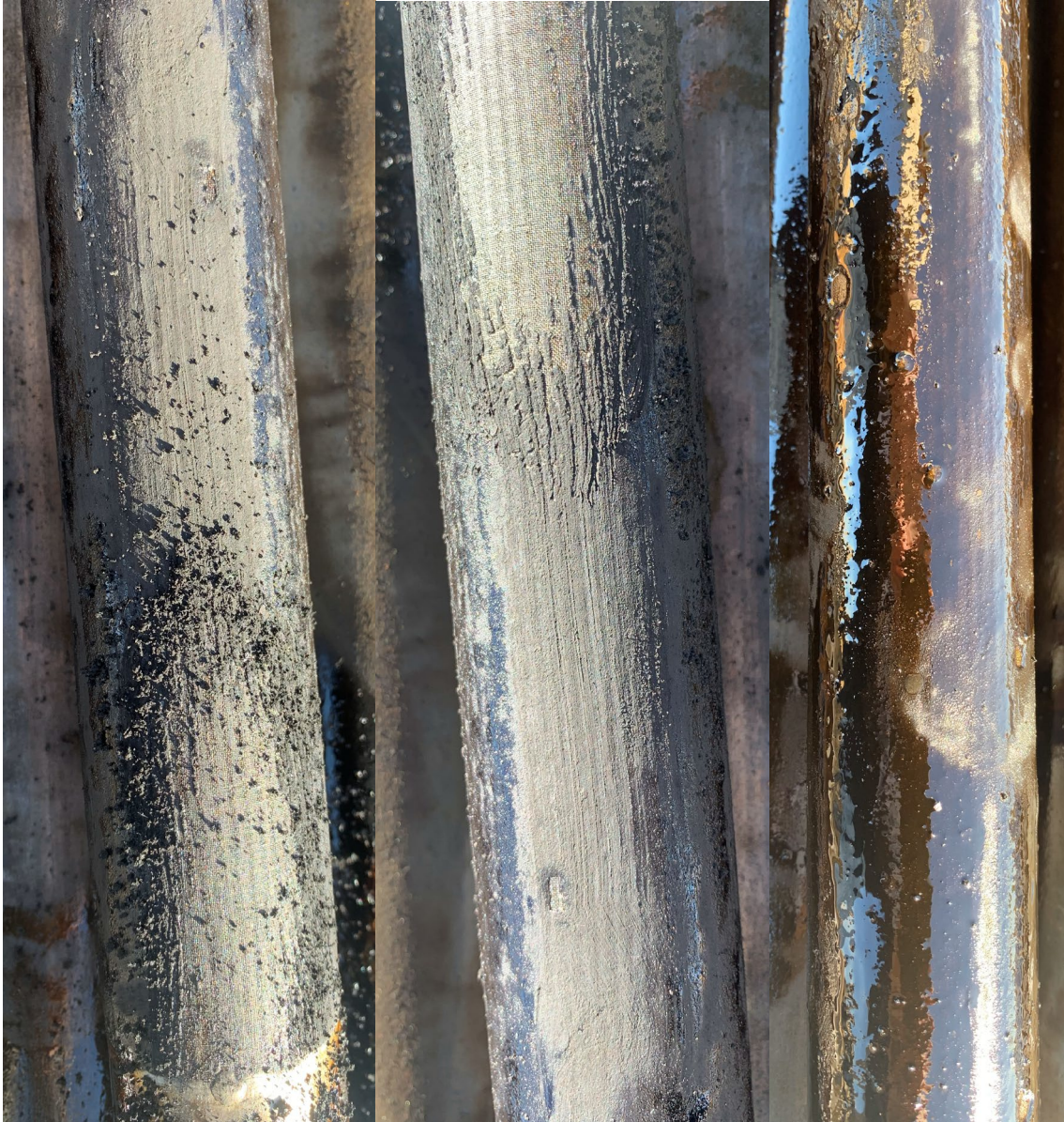
FIGURE 31 – CASE STUDY #3, PLUGGED FILTERING SCREENS, NO BFSV USED
