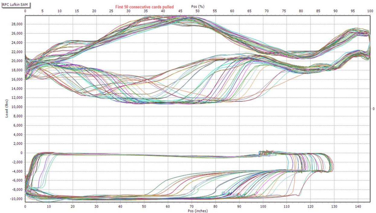
**FIGURE 12 – ANNULAR FLUID LEVEL ABOVE TAC, UNSTABLE FLOW AND PUMP FILLAGE**
