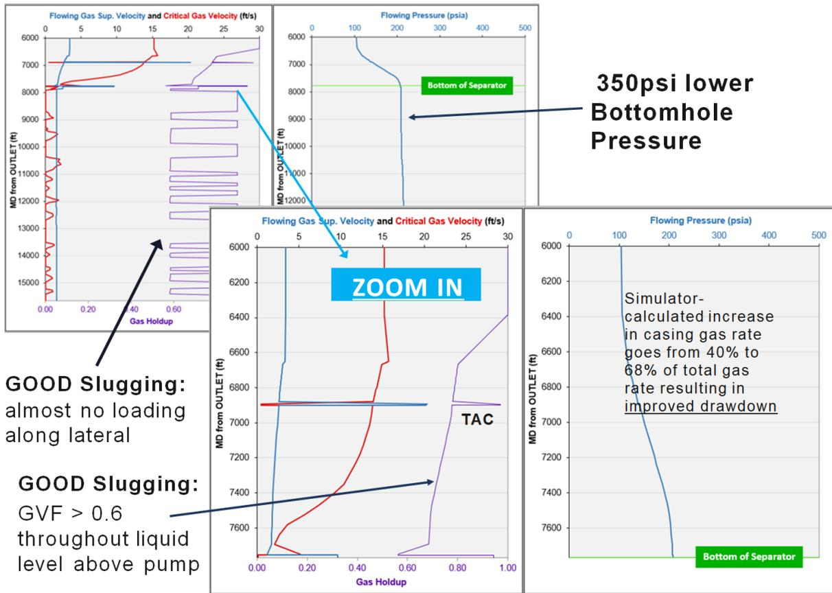
**FIGURE 21 – CASE STUDY #1, FLOW MODELLED PUMP IN CURVE SYSTEM**
