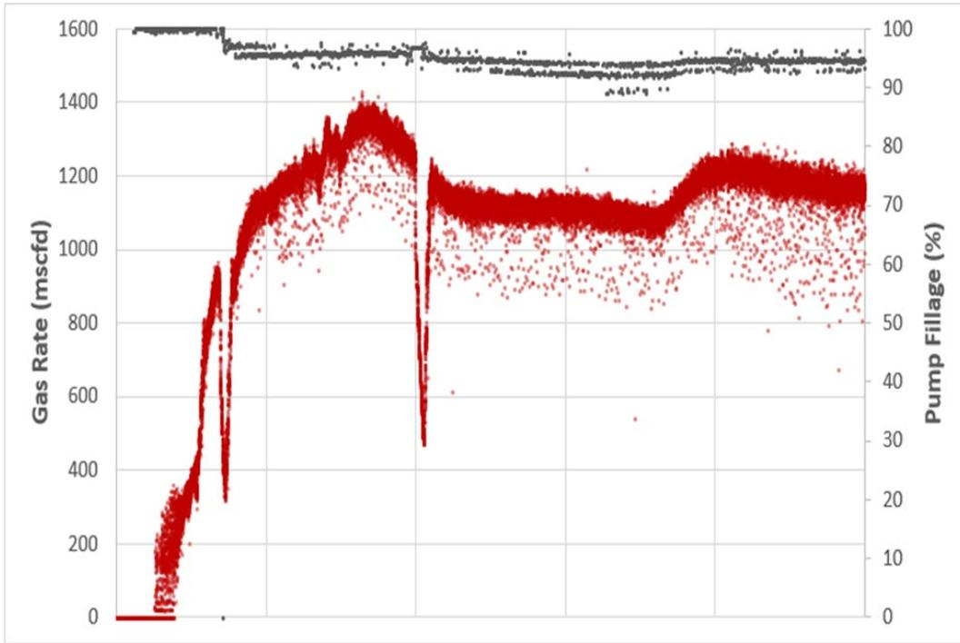
**FIGURE 29 – CASE STUDY #2, STABLE FLOW CONDITIONS AND CONSISTENT HIGH PUMP FILLAGE**
