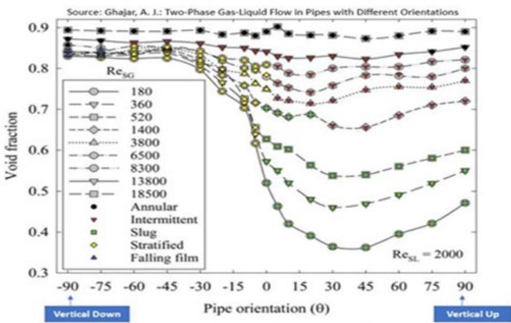
FIGURE 10 – EFFECT OF INCLINATION ON GAS VOLUME FRACTION
