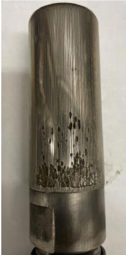
**FIGURE 25 – CASE STUDY #1, FAILED PUMP PLUNGER WEAR**
