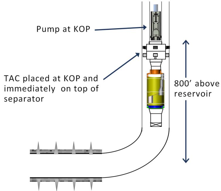
**FIGURE 1 – PUMP PLACED ABOVE THE WELLBORE CURVE**
