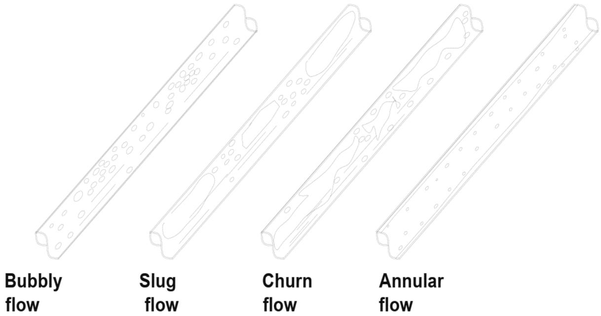
FIGURE 9 – FLOW PATTERNS OR REGIMES AT INCLINATIONS
