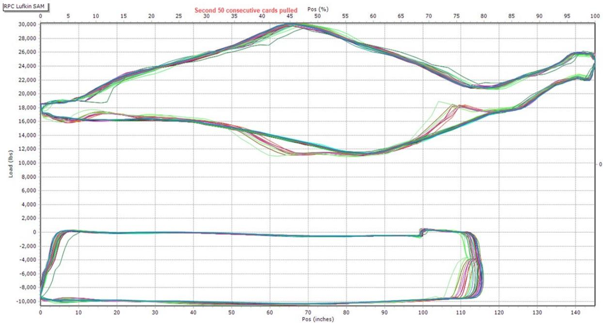
**FIGURE 13 – ANNULAR FLUID LEVEL BELOW TAC, STABLE FLOW AND PUMP FILLAGE**
