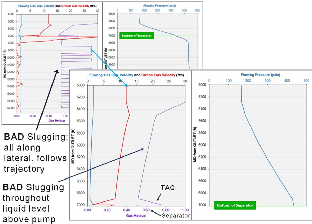
**FIGURE 26 – CASE STUDY #2, FLOW MODELLED PUMP ABOVE KOP WITH SLIMHOLE TAC**
