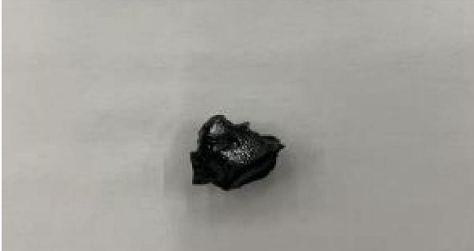
**FIGURE 24 – CASE STUDY #1, DEBRIS IN PUMP FAILED STANDING VALVE**
