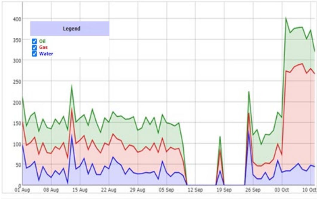
**FIGURE 11 – PRODUCTION UPLIFT FROM REMOVAL OF RESTRICTIVE TAC AND INSTALLING A HIGH PERFORMANCE LIQUID FALLBACK SEPARATOR**
