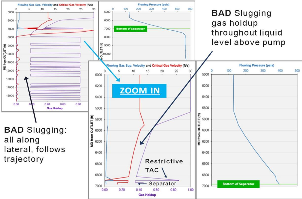
**FIGURE 19 – CASE STUDY #1, FLOW MODELLED PUMP ABOVE KOP WITH RESTRICTIVE TAC**
