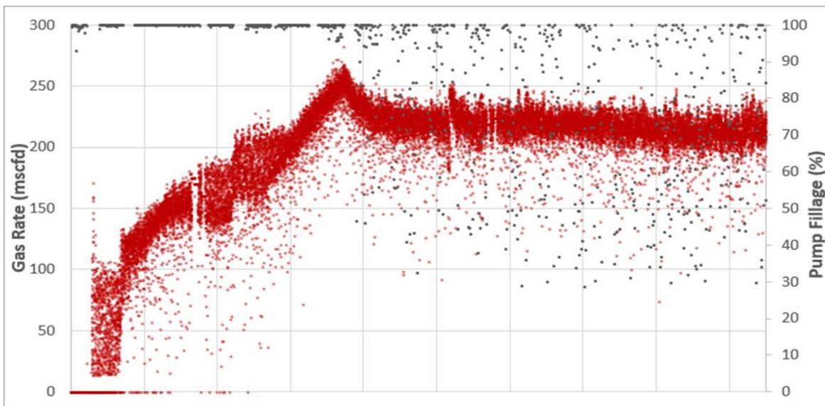
**FIGURE 22 – CASE STUDY #1, STABLE FLOW CONDITIONS AND CONSISTENT HIGH PUMP FILLAGE**
