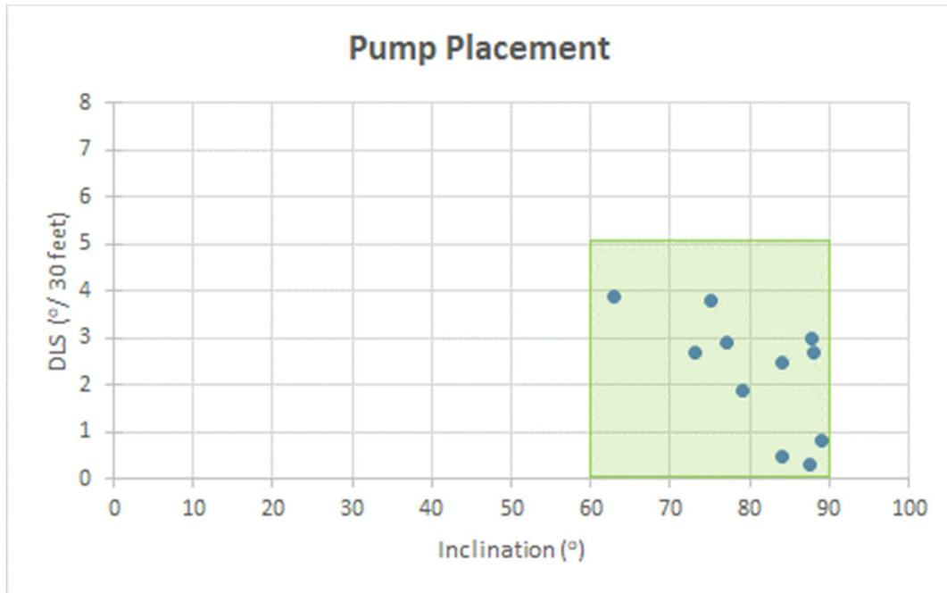
**FIGURE 5 – CASE STUDY SUMMARY OF PUMP PLACEMENTS INCLINATIONS**
