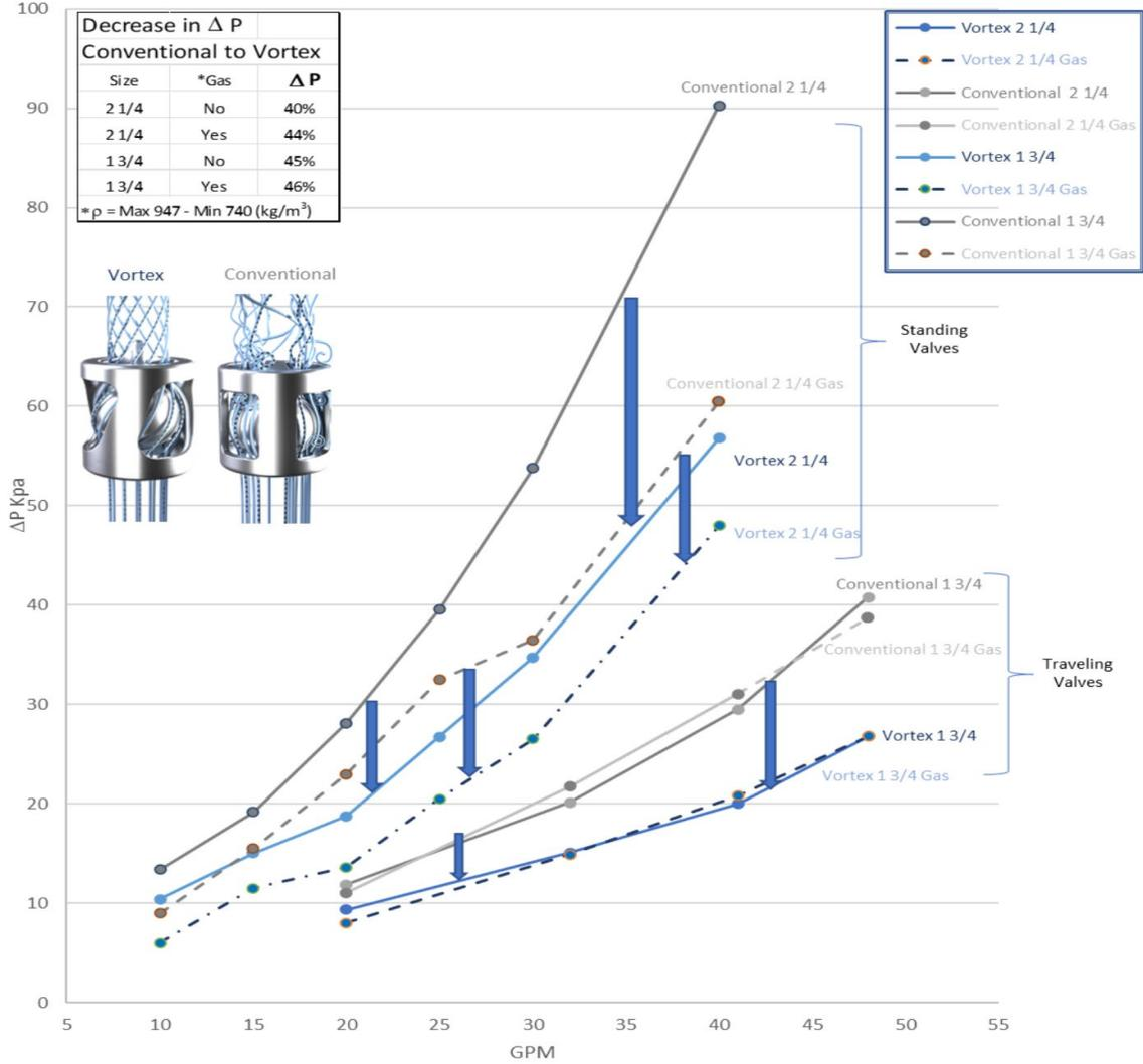
**FIGURE 17 – Q2 FLOW VORTEX FLOW PUMP VALVES REDUCE FLUID FLOW PRESSURE LOSS**
