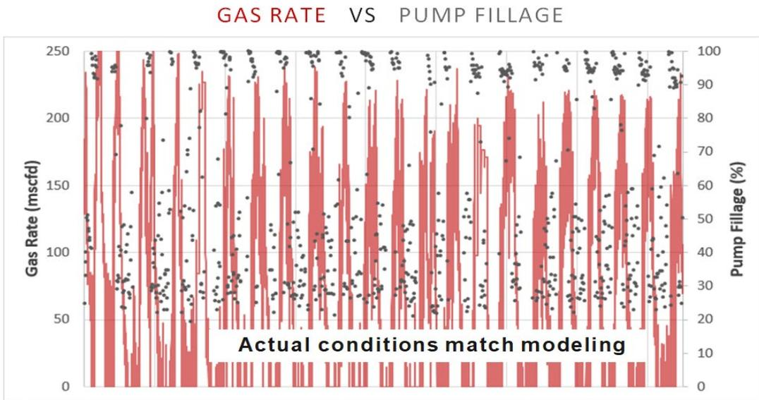
**FIGURE 20 – CASE STUDY #1, UNSTABLE FLOW CONDITIONS AND POOR ERRATIC PUMP FILLAGE**
