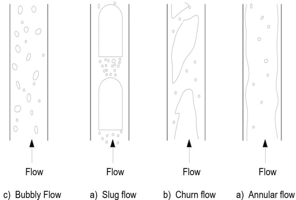
**FIGURE 8 – FLOW PATTERNS OR REGIMES AT VERTICAL INCLINATION**
