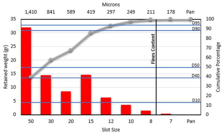
Figure 1 sieve set up and granulometric distribution.
