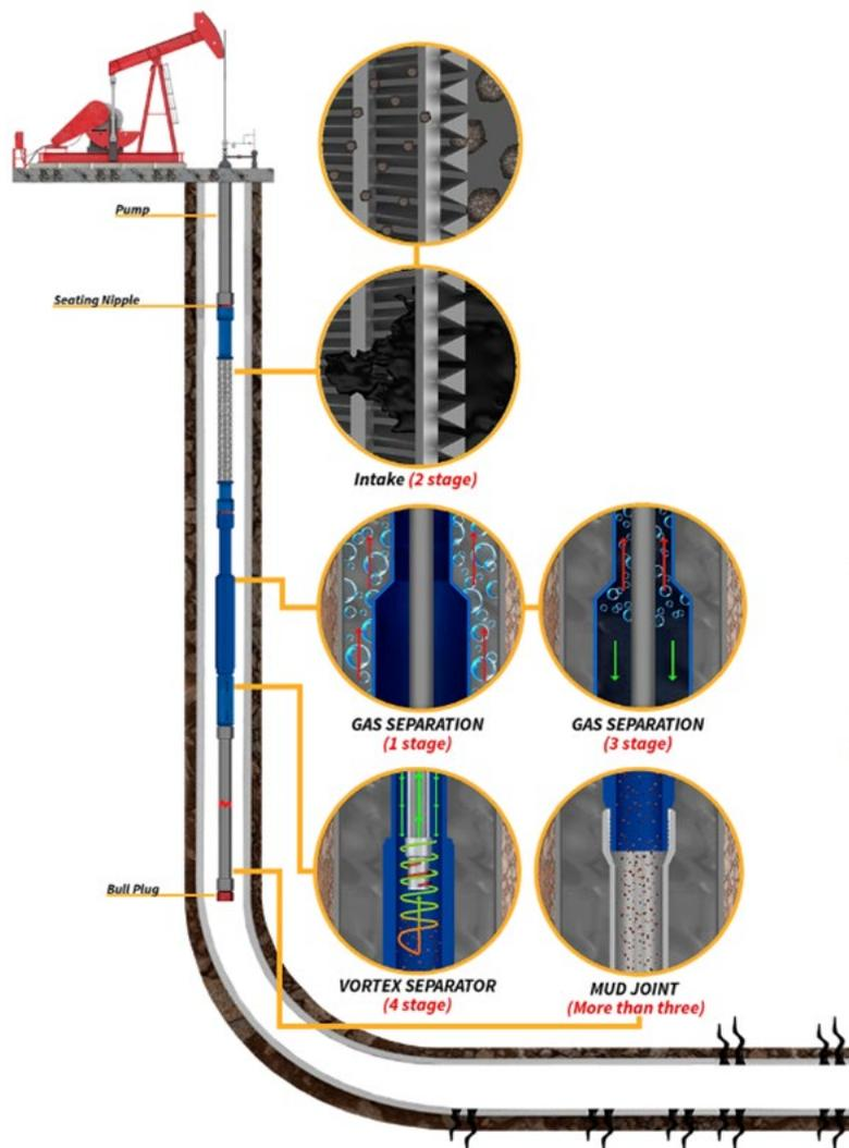
Figure 2 Combination Tool: 2-Stage Filtration with Gas Separation
