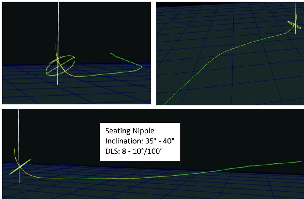
Figure 3 Deviation sketch of the wells designed.
