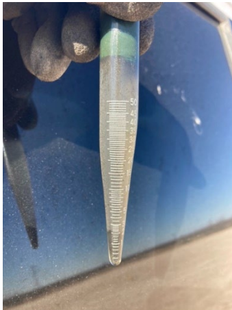
(a) Post-Workover-Iron Sulfide deposits
