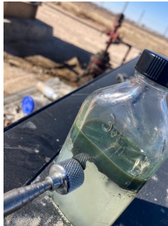
(b) Post-Workover- Iron Sulfide-magnetic
