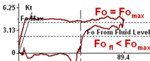
Figure 16 – Pump dynamometer characteristics of three causes of incomplete pump fillage and relationship to fluid level surveys.
