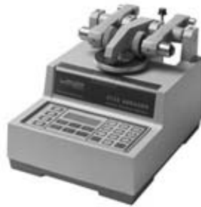
Figure 4 – Example Tabor Abraser Device
