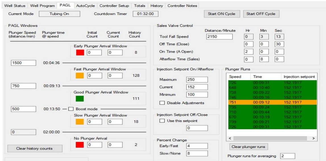
Figure 3 PAGL Optimization in Horizontal STACK Well (Series 8000™ Controller)
