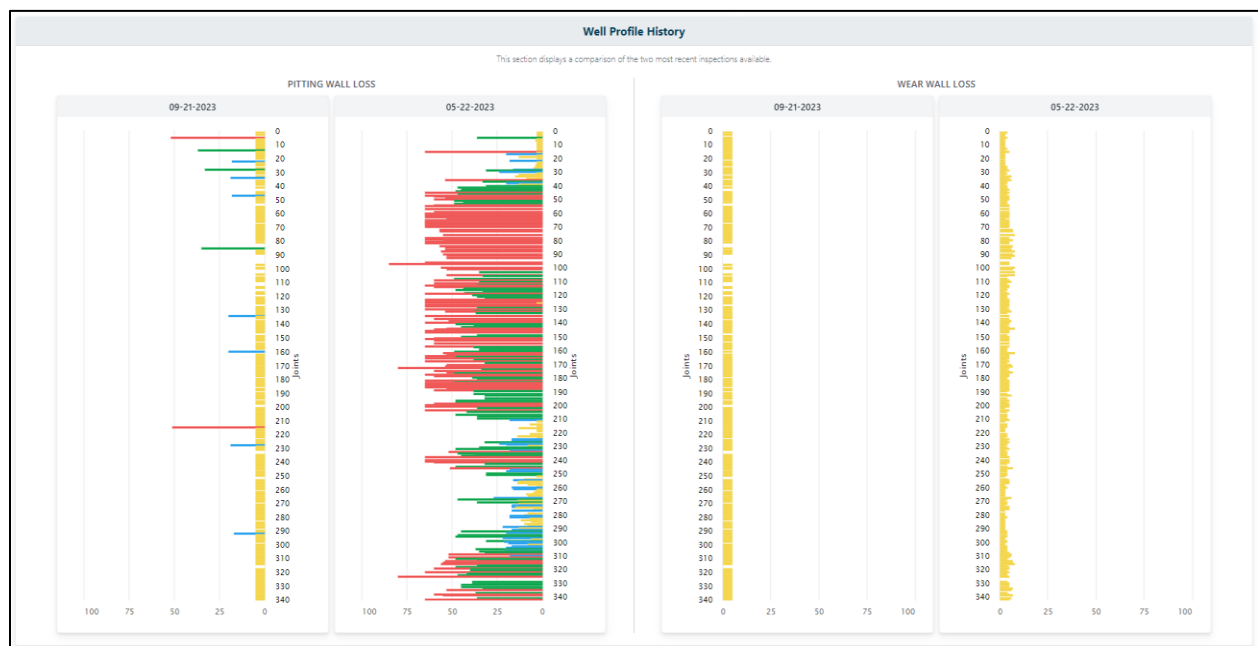
Figure 6 – Side-by-side inspection results for the same well taken at different points in time.
