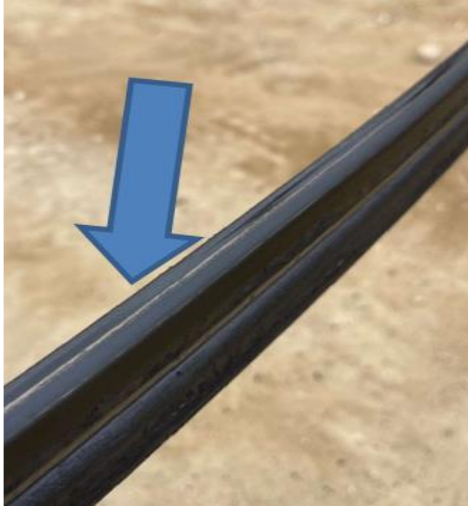
Figure 17: Well No. 4 - Wear on Minor
