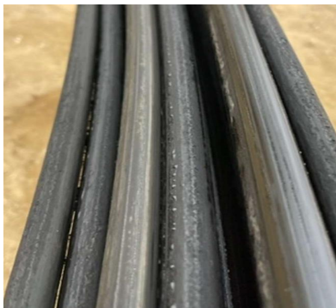
Figure 16: Well No. 4 - Moderate to Severe Scale Pitting
