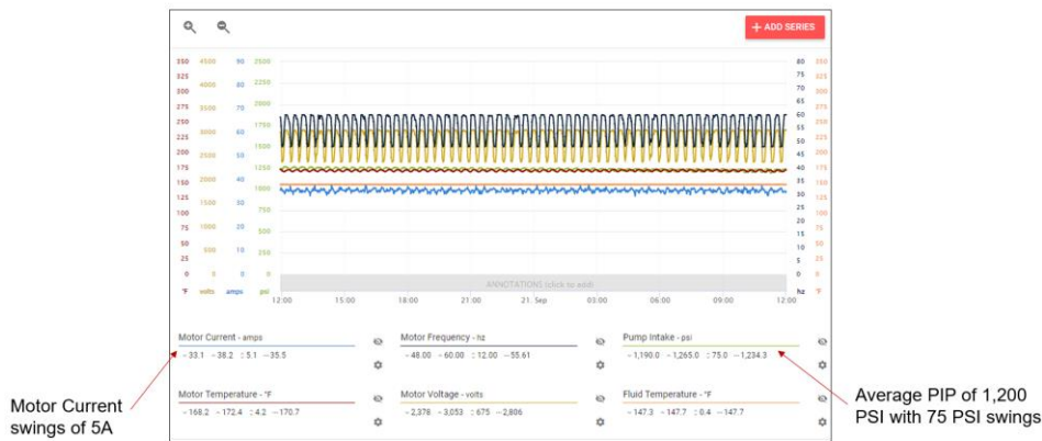
Figure 7 - Single Hydro-Helical Slugger Gas Separator performance in slugging conditions at approximately 1,200 PIP.
