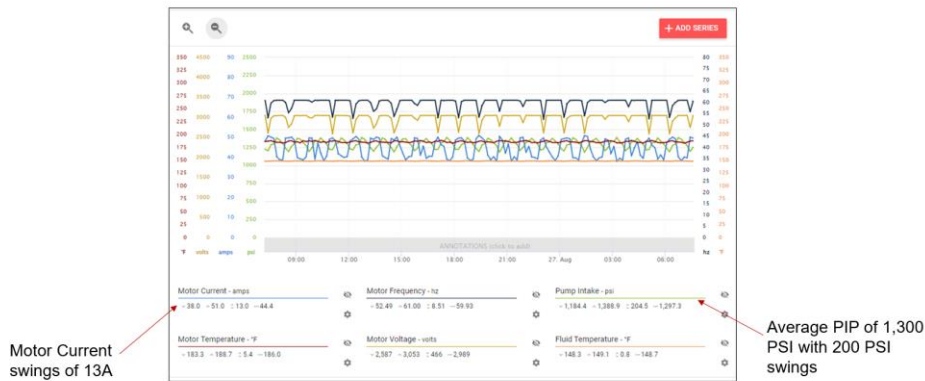
Figure 6 - Tandem Hydro-Helical Gas Separator performance in slugging conditions at approximately 1,300 PIP.
