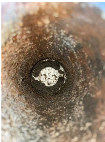
Figure 6 Sand accumulation inside the tool
