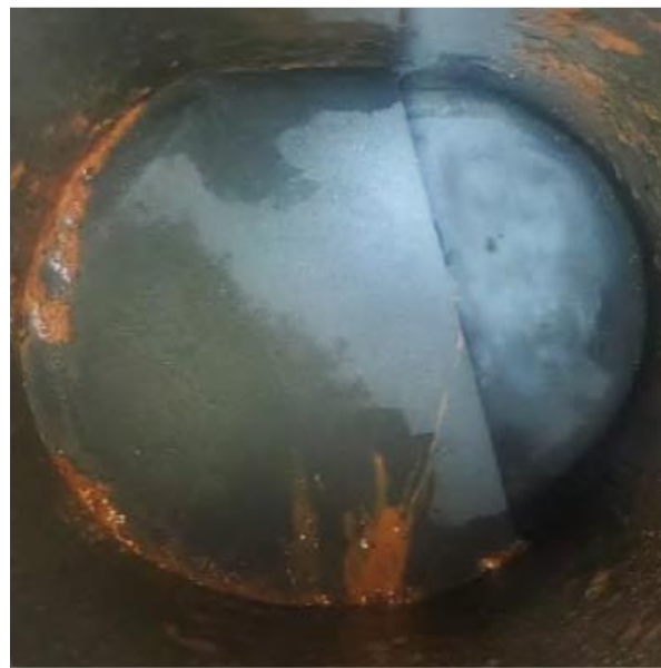
Figure 10: Deflector Plate, after Erosion Test
