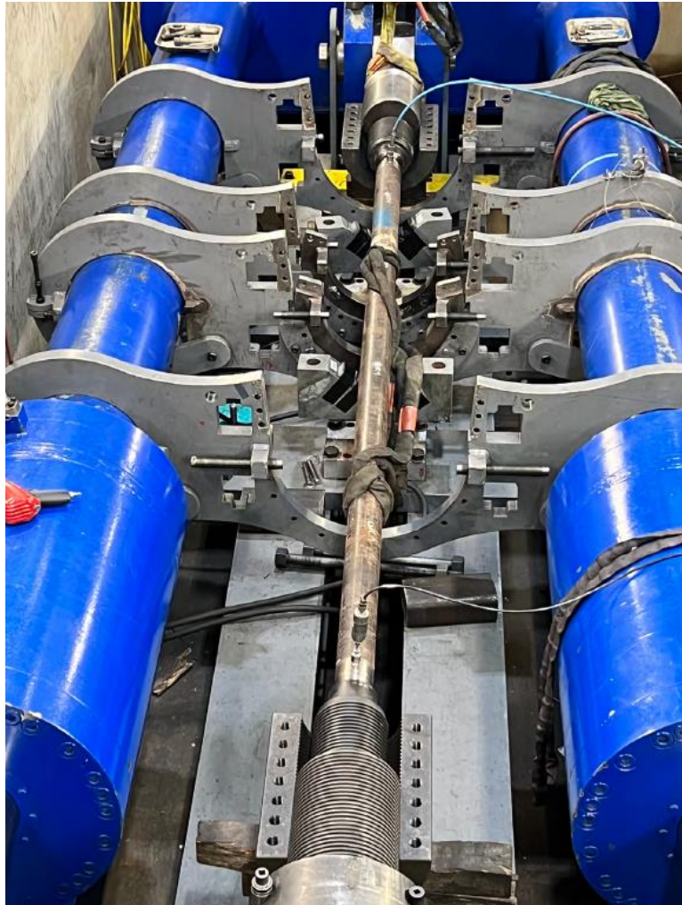
Figure 12: Tensile and Compression Proof Load Test Setup
