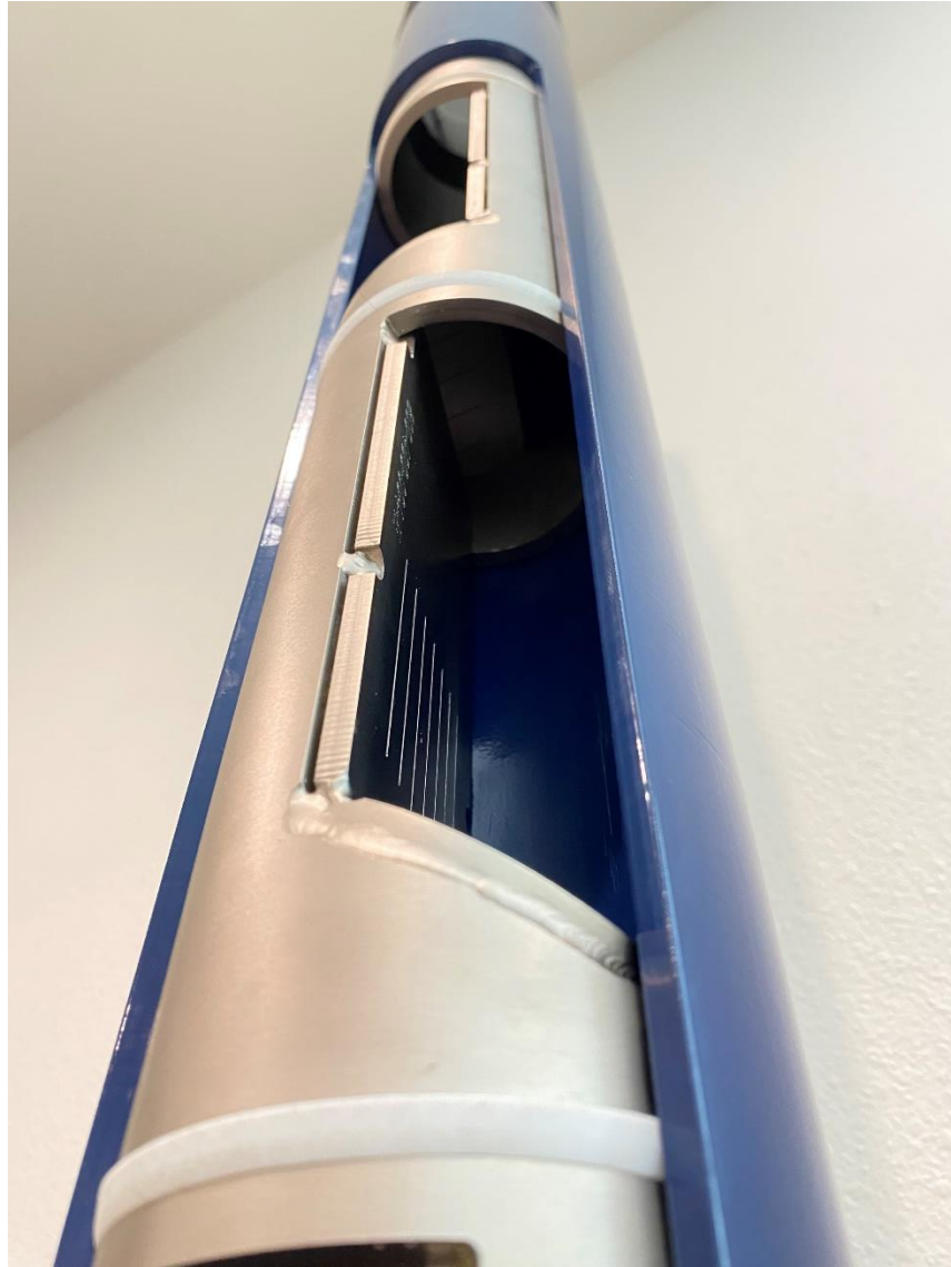
Figure 3: Cut-away Side Profile showing Flow Path through tool
