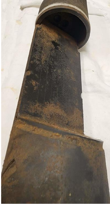
Figure 16: Chamber showing no erosion, only surface rust from Field Test
