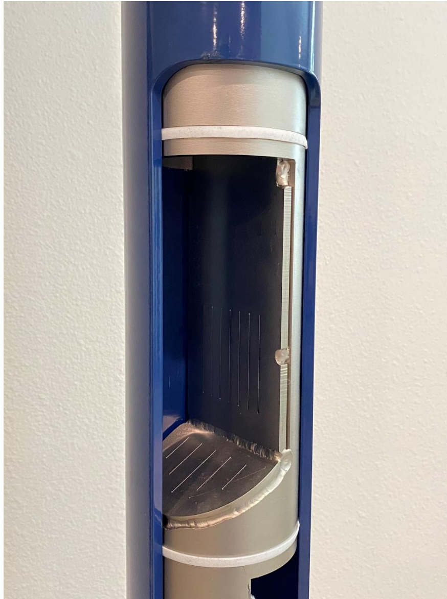
Figure 2: Cut-away Side Profile of one of the Sand-Bearing Chambers
