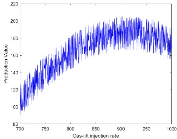
Figure 3: Gas Lift Performance Curve with noise
