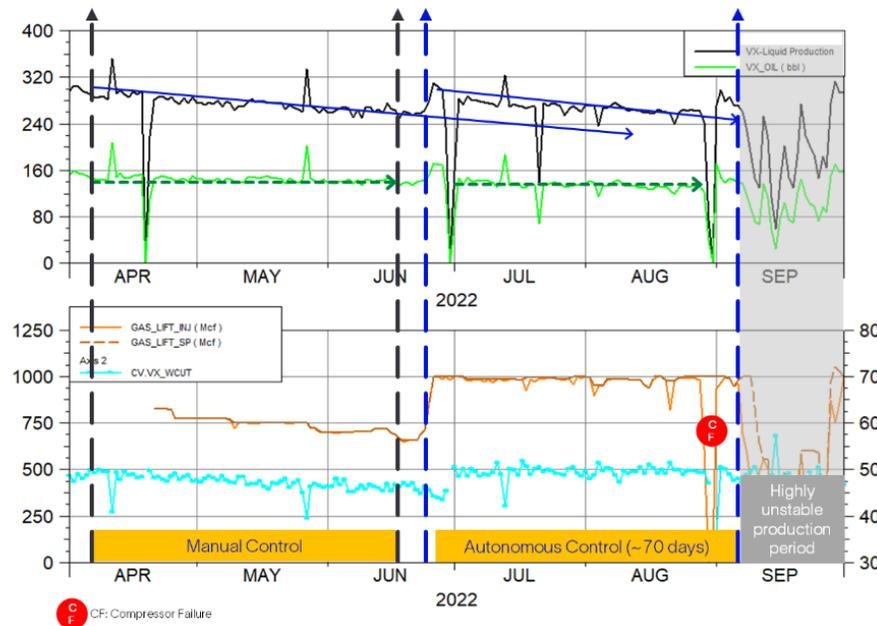
Figure 11: Well 2 production profile showing before and after DD GLO implementation.
