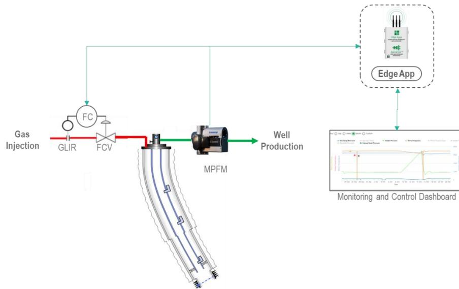
Figure 6: Example of field installation
