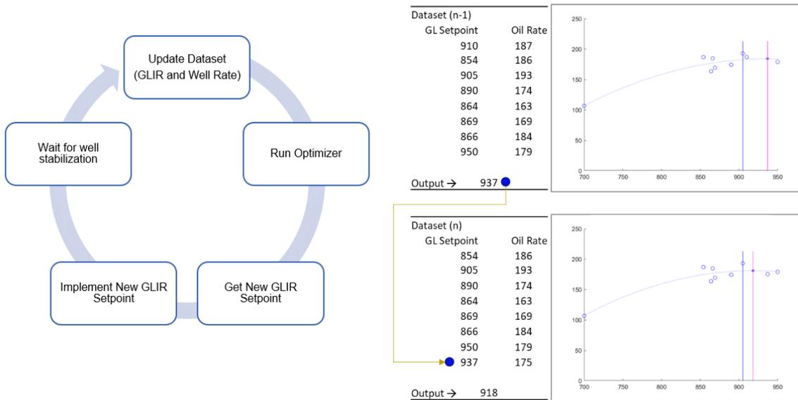
Figure 5: Data-Driven Gas Lift Optimization process
