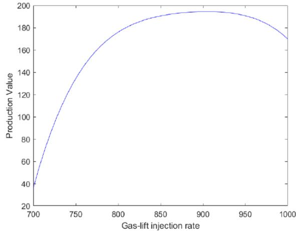
Figure 1: Gas Lift Performance Curve without noise
