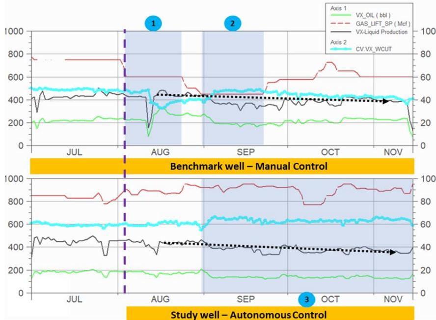
Figure 8: Application adaptation example to changes on water-cut vs manual operation.
