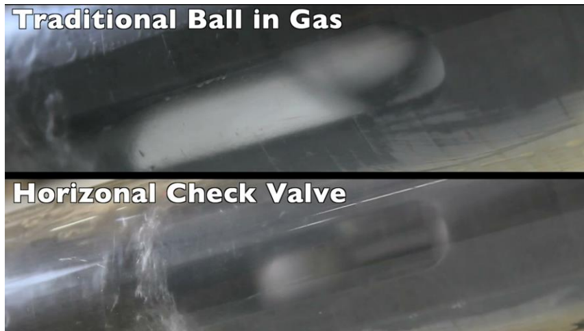
Figure 5 Flow testing comparison in gas
