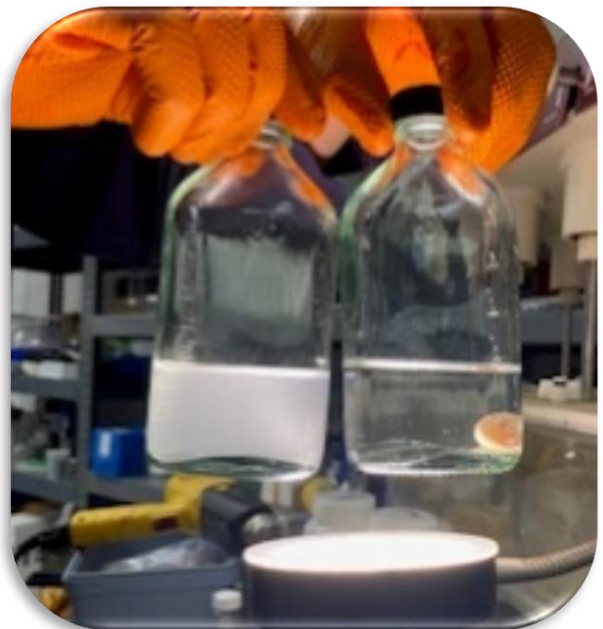
Figure 3B: Homogeneous microencapsulated matrix concept: from left to right: (a) calcium carbonate scale formation under heating, with no microencapsulated scale inhibitor (b) calcium carbonate scale inhibition, with Microencapsulated scale inhibitor.
