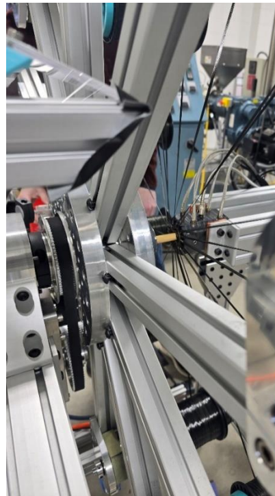
FIGURE 15 – RADIAL TORQUE WRAPPING AN FRTP ROD FOR INCREASED TORQUE CAPACITY
