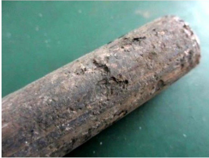
FIGURE 3 – STEEL SUCKER ROD CORROSION AND CORROSION RELATED FATIGUE FAILURE
