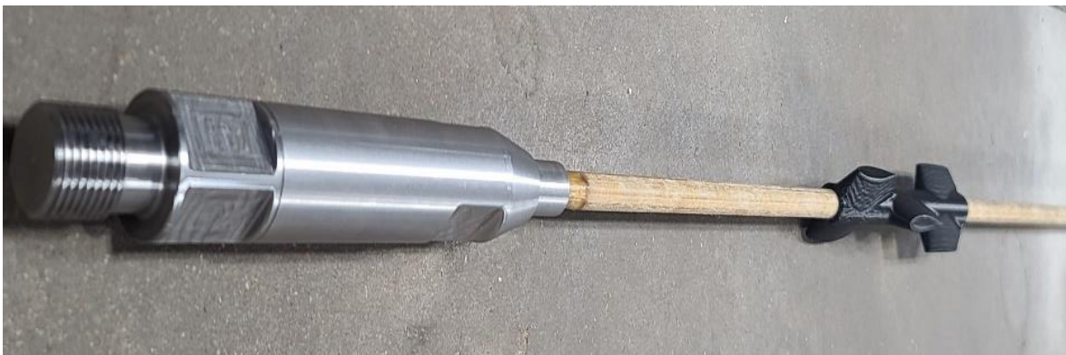
FIGURE 26 – STAGE 3 OF MANUFACTURING: INSTALLATION OF THERMOPLASTIC ROD GUIDES AND METAL END FITTINGS
