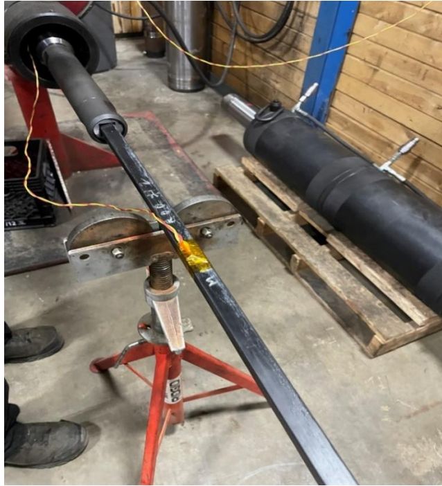
FIGURE 31 – EXAMPLE FRTP SUCKER ROD TEMPERATURE AND CREEP LOAD TESTING
