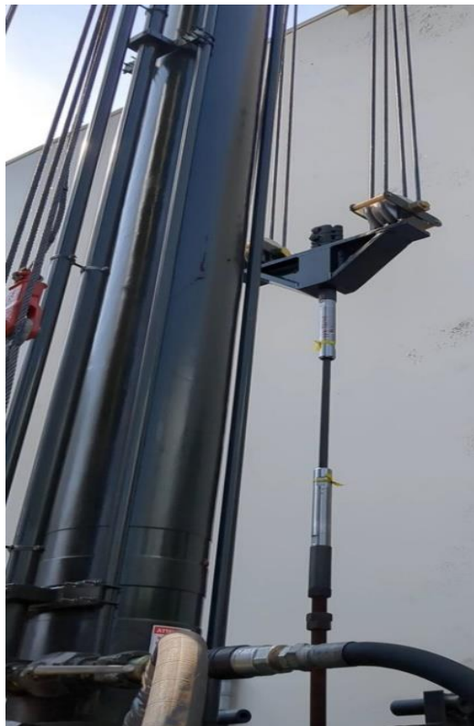
FIGURE 32 – EXAMPLE FRTP SUCKER ROD AND END FITTING FATIGUE TESTING (SSI CALGARY YARD)
