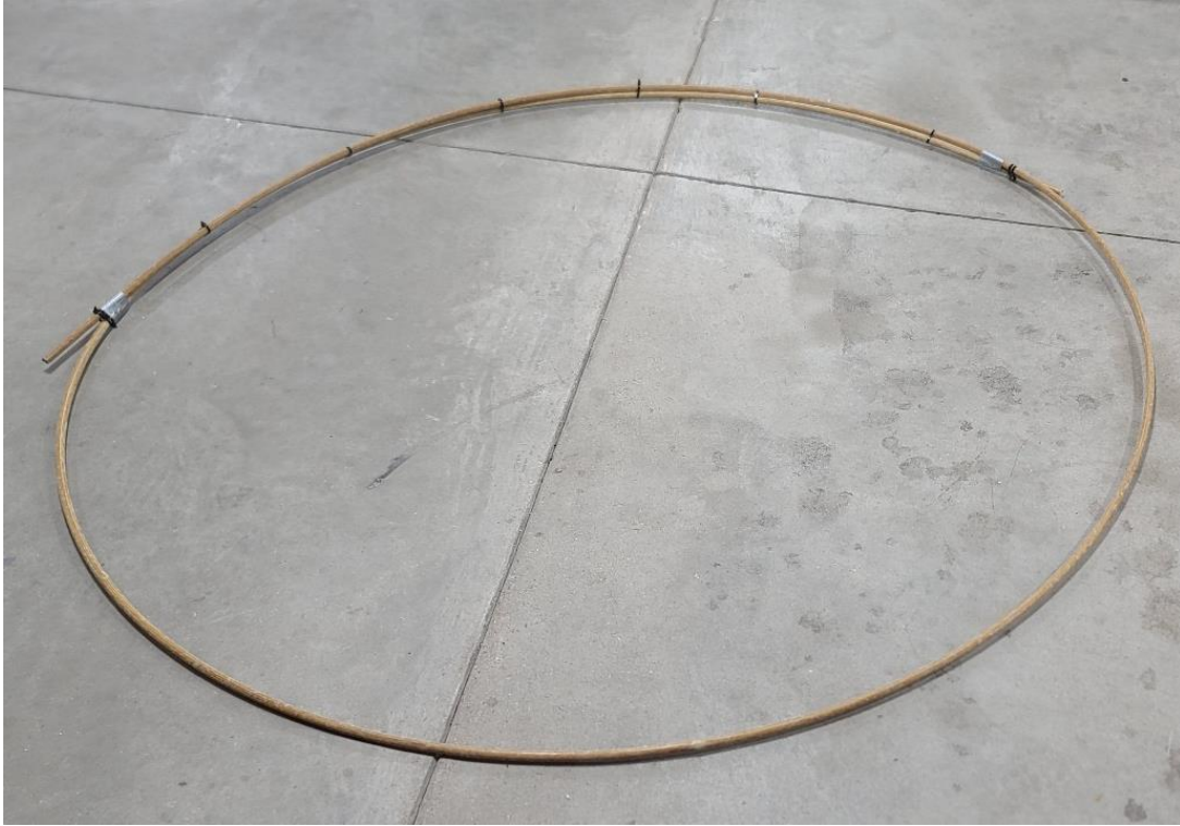
FIGURE 11 – COILED FRTP SUCKER ROD, DEMONSTRATING HIGH SHEAR FAILURE TOLERANCE
