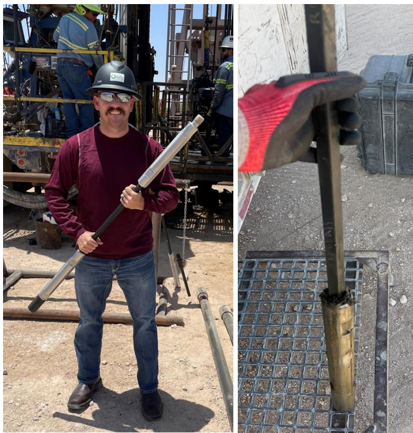
FIGURE 43 – SUCCESSFUL FRTP PONY SUCKER ROD PERMIAN WELL TRIAL
