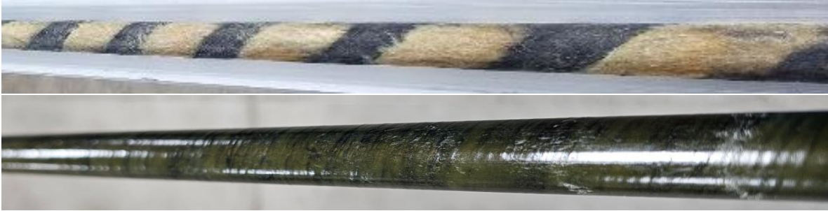
FIGURE 16 – RADIAL TORQUE WRAPPED FRTP RODS
