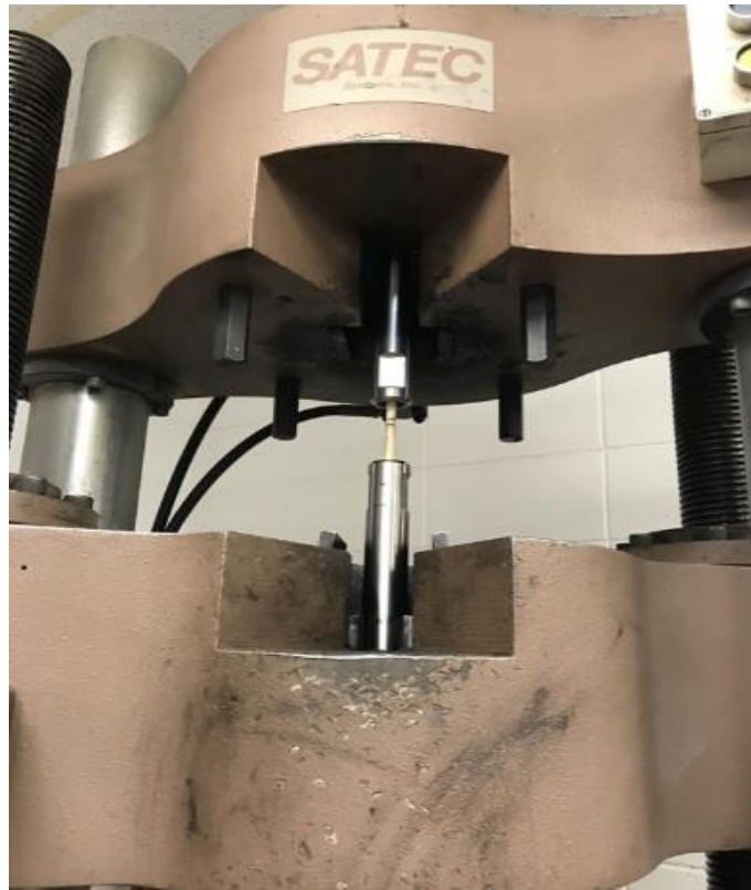
FIGURE 29 – FRTP SUCKER ROD AND END FITTING TENSILE TESTING APPARATUS.
