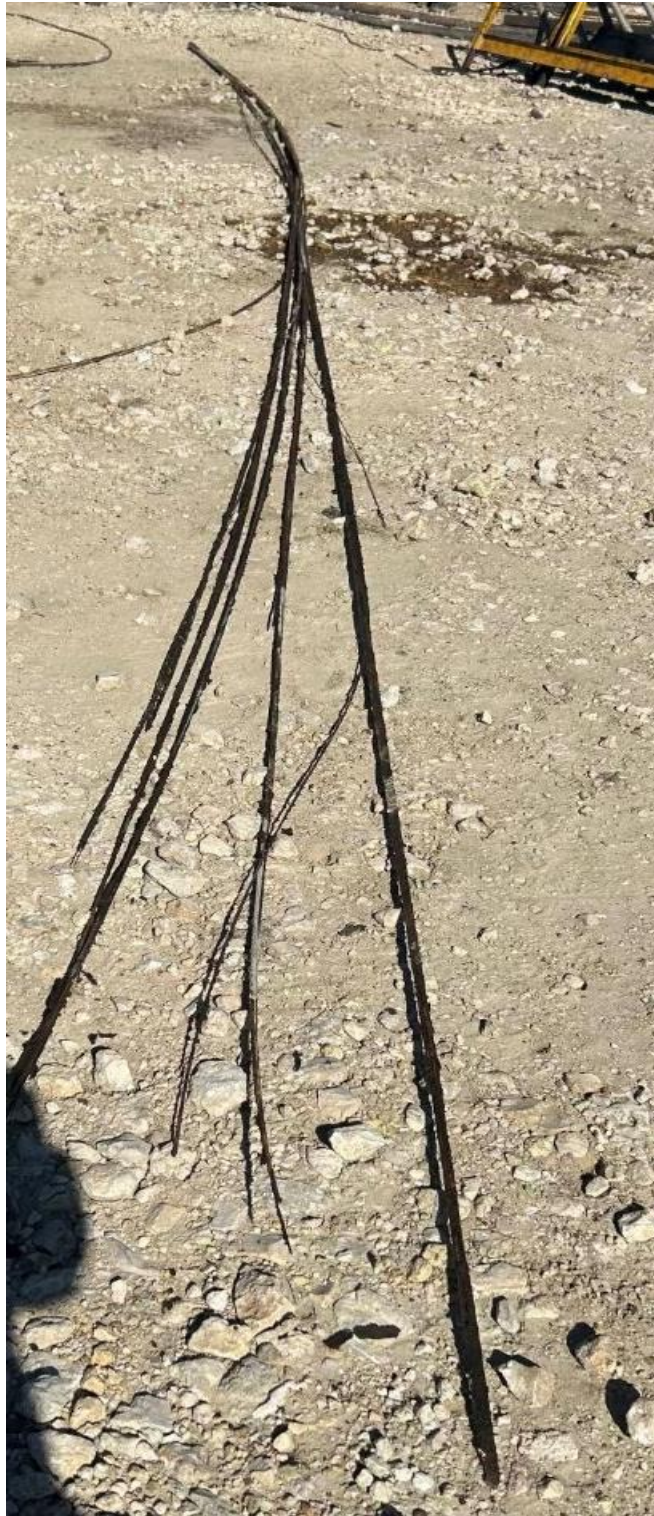
FIGURE 33 – EXAMPLE THERMOSET FIBERGLASS SUCKER ROD FAILURE AND “BROOM STICKING” FAILURE MECHANISM.
