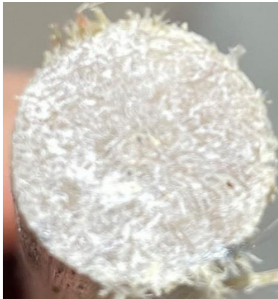
FIGURE 25 – ADEQUATELY CONSOLIDATED FRTP ROD
