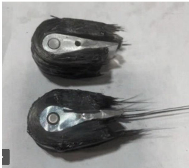
FIGURE 20 – THERMOPLASTIC FIBER ORIENTATION STRESS CONCENTRATION FAILURE IN AN EARLY-PHASE PROTOTYPE END FITTING
