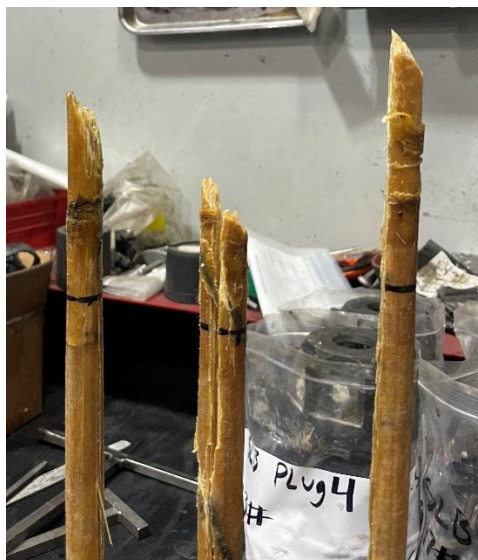
FIGURE 36 – FRTP FAILURE TESTING UNDER TENSILE LOADING
