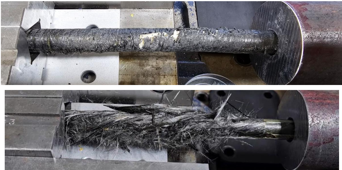
FIGURE 18 – FRTP ROD TORQUE FAILURE TESTING
