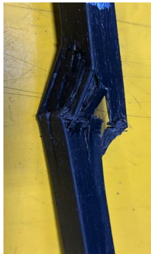
FIGURE 35 – FRTP FAILURE TESTING UNDER COMPRESSIONAL LOADING
