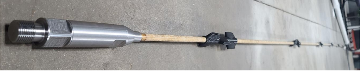
FIGURE 39 – COMPLETE FRTP SUCKER ROD
