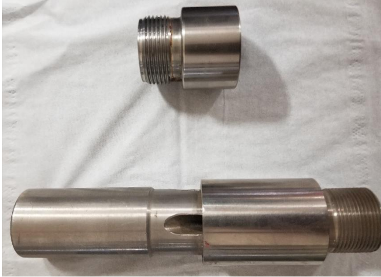
Figure 10 shows an example of the external seat plug and top plunger adapter used in Sand Diverter pump applications
