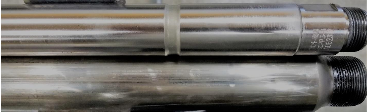
Figure 5 shows the difference between a grooved (Top) and smooth body plunger.
