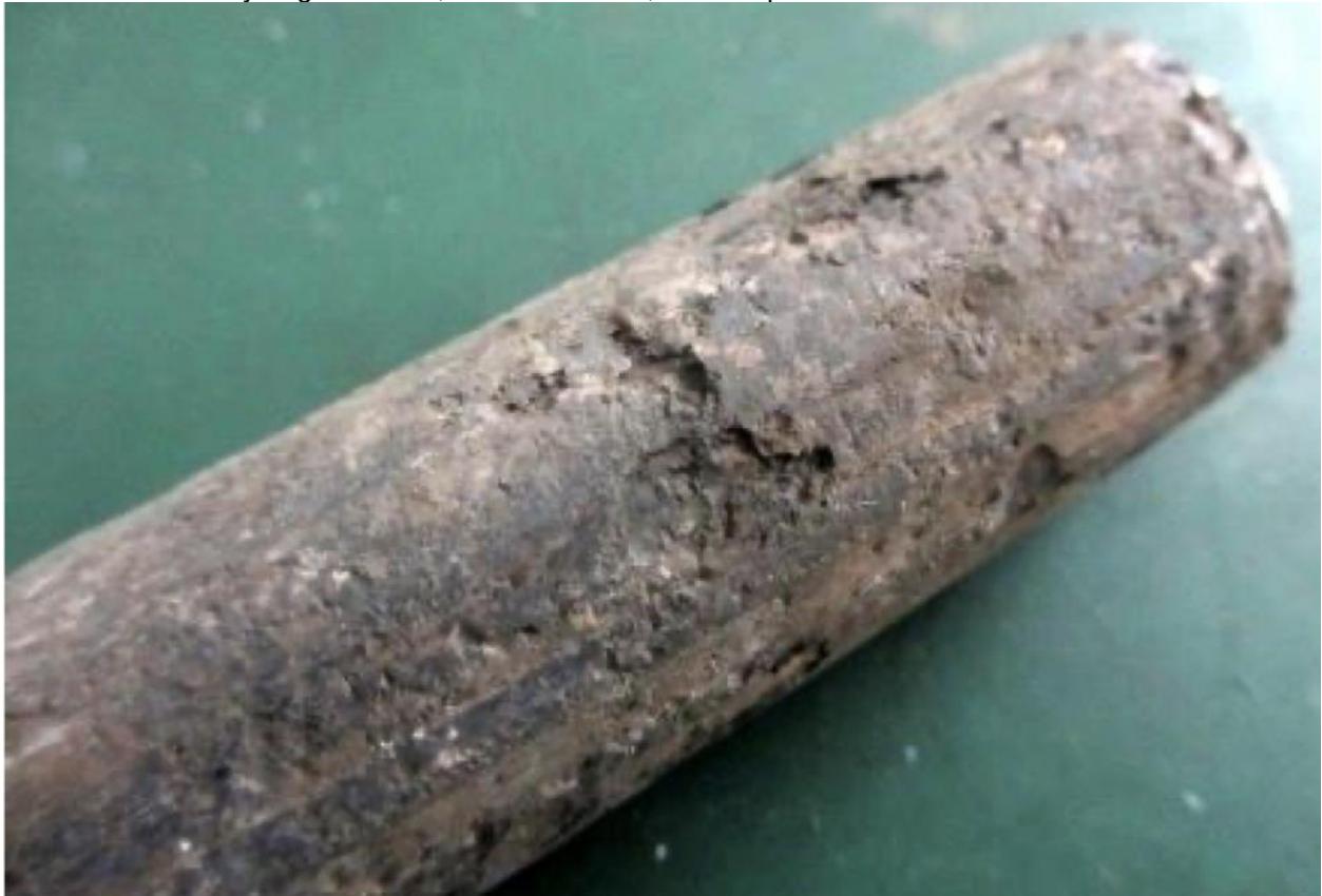
Figure 2 – Localized Corrosion Morphology (Zhang et al.)
