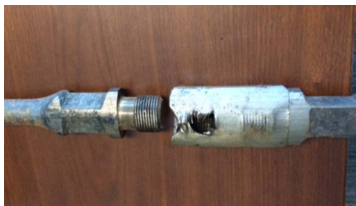
Figure 3 - Rod pin pulled out of worn coupling
