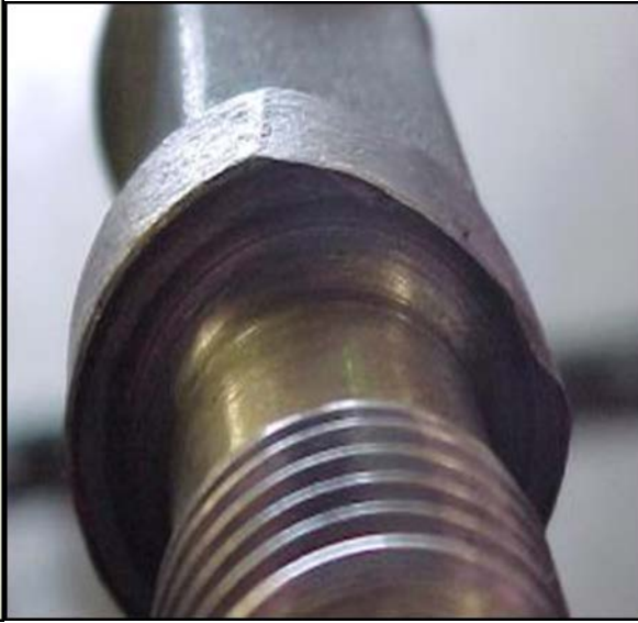
Figure 5 - Worn rod shoulder
