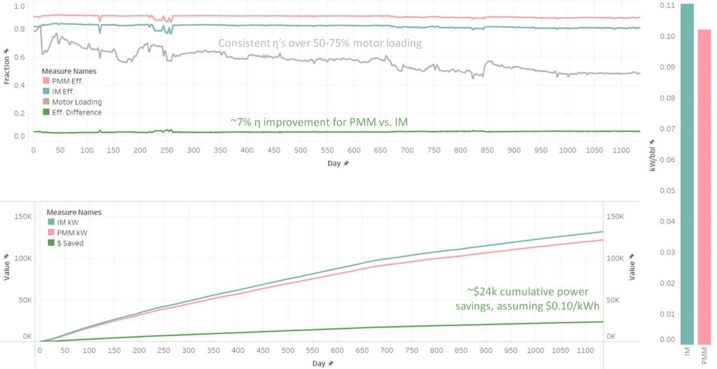
Figure 13 – Unconventional consolidated motor  $\eta$  and loading (top), cumulative power and savings (bottom), and calculated power per unit of liquid lifted (right).
