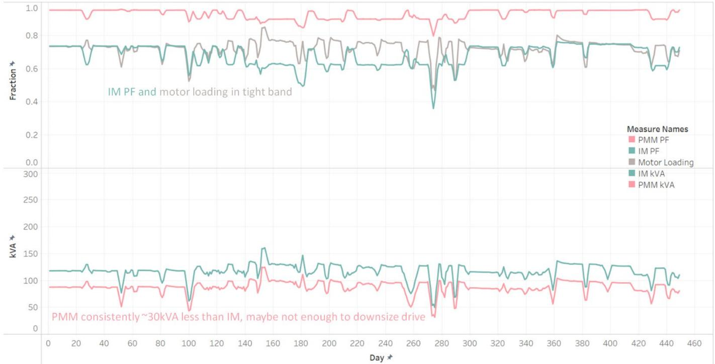
Figure 18 – Conventional consolidated motor PF and loading (top) and kVA usage (bottom).
