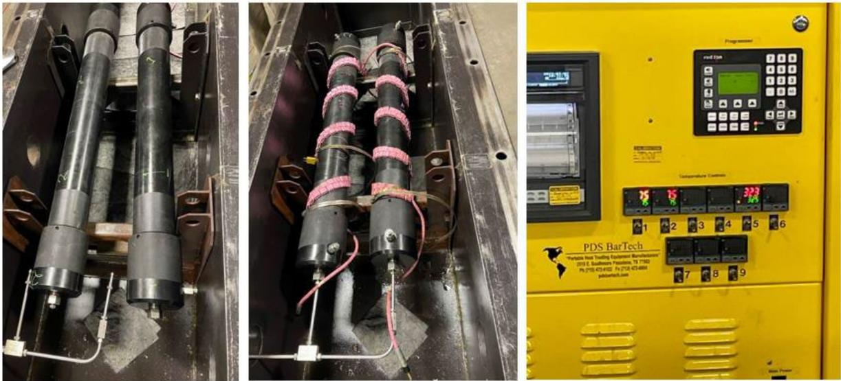
Figure 9 – Valves for Test Loaded into Their Respective Chambers
