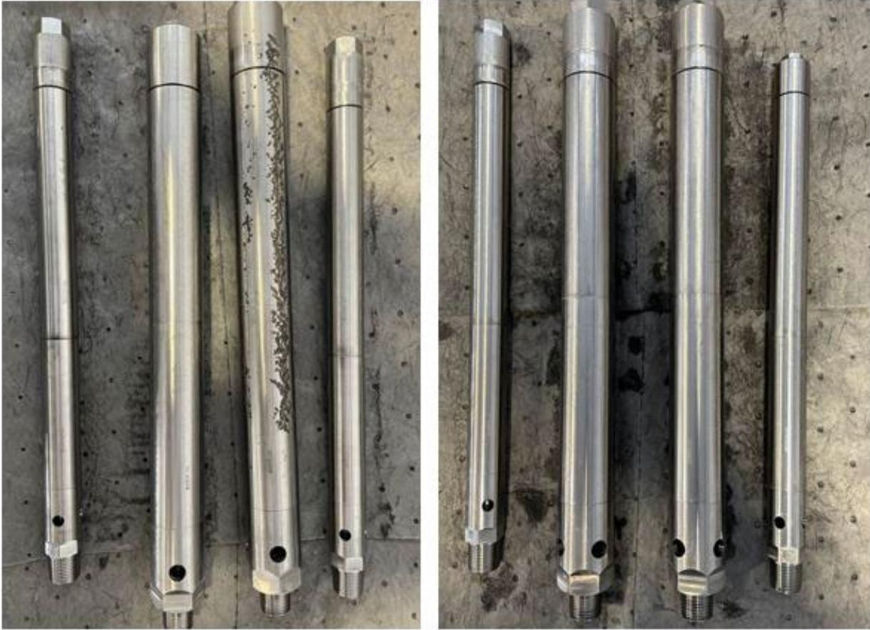
Figure 11 – Valves After Removal from Their Respective Testing Chambers
