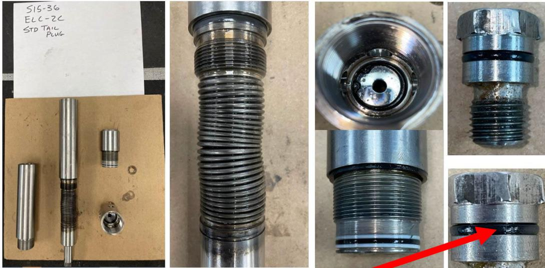
**Evidence of Elastomer Degradation Found**
