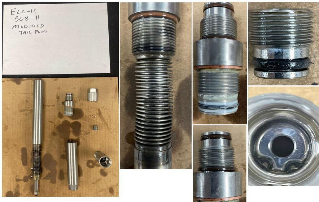
Figure 13 - Elastomer Condition of 1.0" Robust Valve Post Testing
