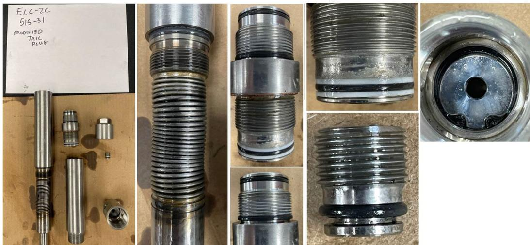
Figure 15 - Elastomer Condition of 1.5" Robust Valve Post Testing
