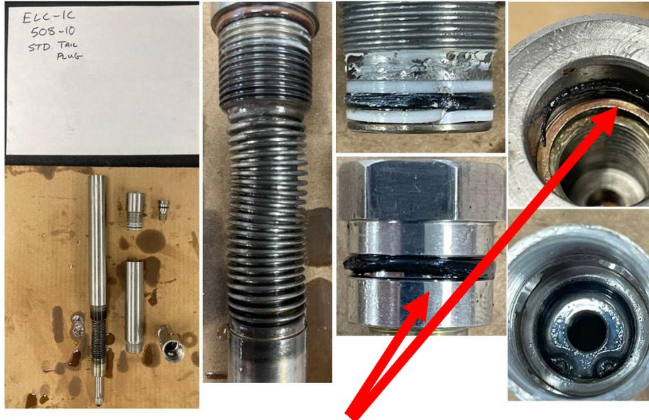
**Elastomer in Very Poor Condition**
